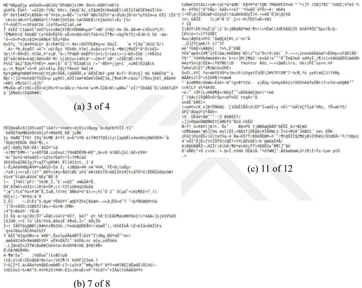
Figure 4.7 Sample faulty extraction results obtained with single missing carriers
