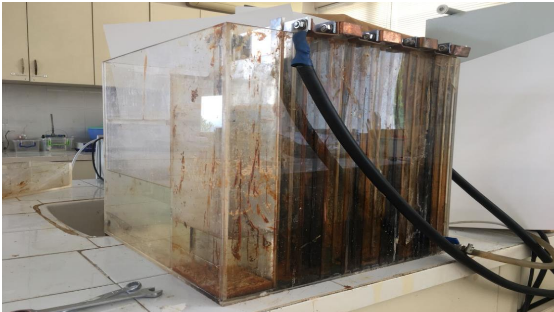
Figure 3.1. Electrode configuration in Electrocoagulation and Electroflocculation reactors.
