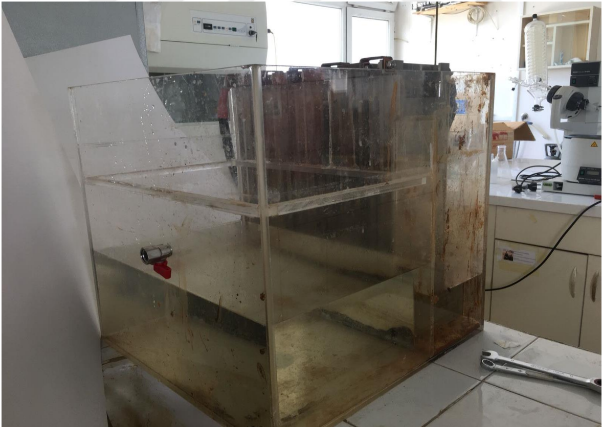
Figure 3.3. Electrocoagulation and Electroflocculation reactors.
