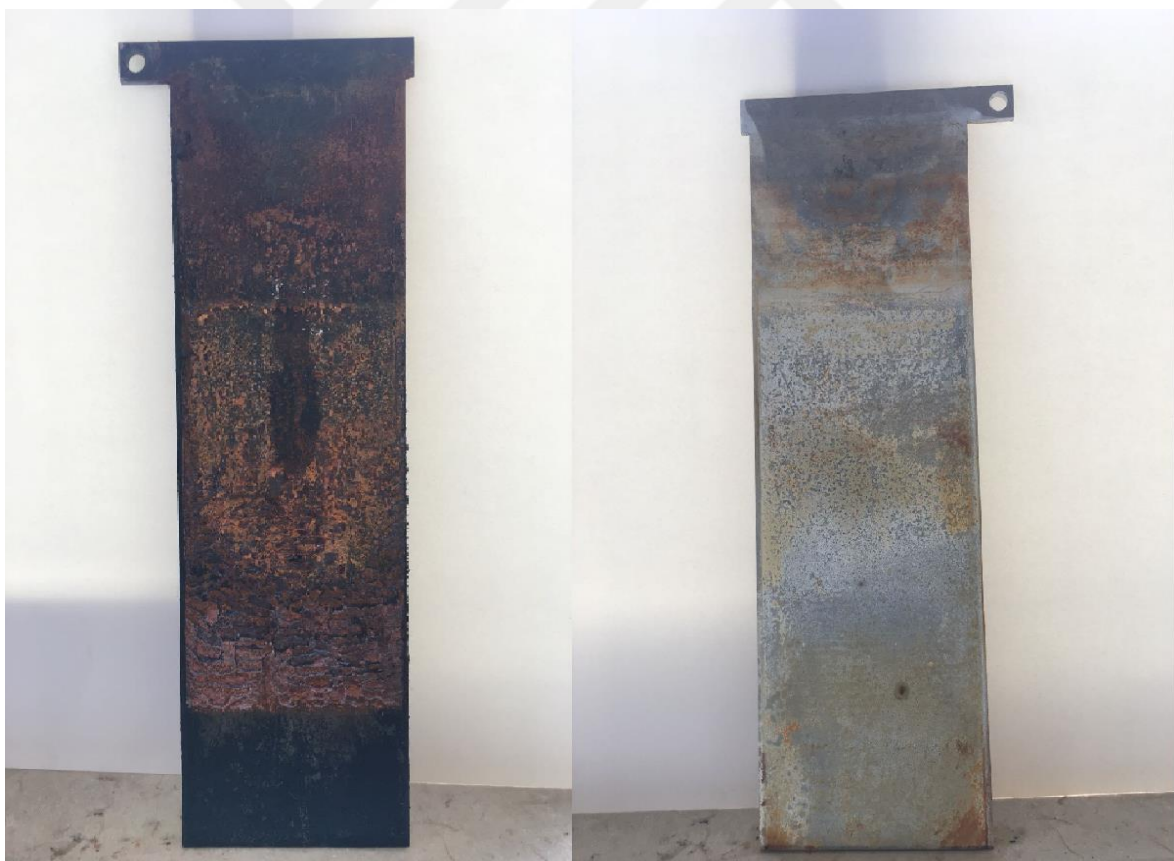
Figure 3.7. Fe and Al electrodes
