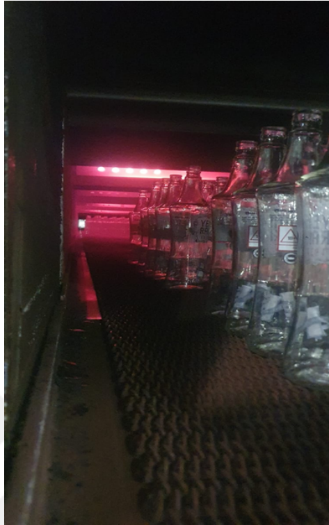
Figure 3.5: A typical annealing furnace viewed from inlet
