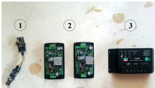
Figure 3.2 Tested MPPTs which are designed for DesTech Solaris Solar Car (1), its telemetry system (1-2), tested commercial MPPT in market.
