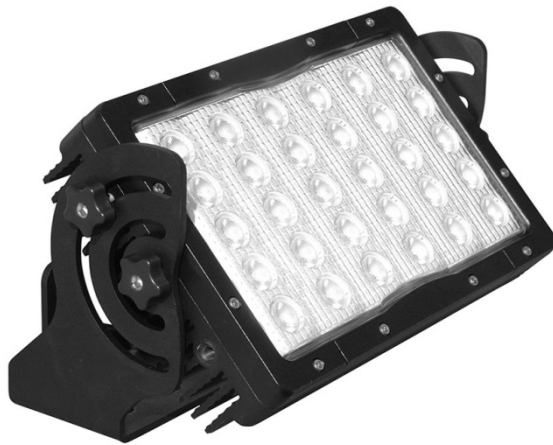
Figure 12: Marine Grade 150 Watt LED Flood Light (10-32 Volts DC, 14,790 Lumens, 12 Ampere)
