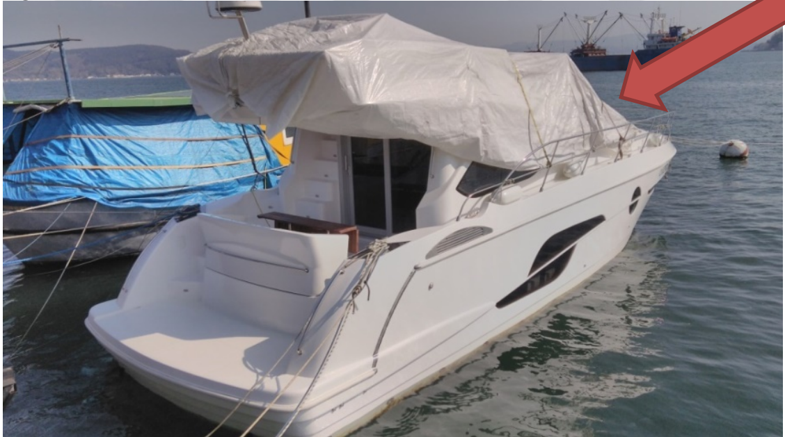
Figure 13: Protection of Boats with Membranes and Covers
