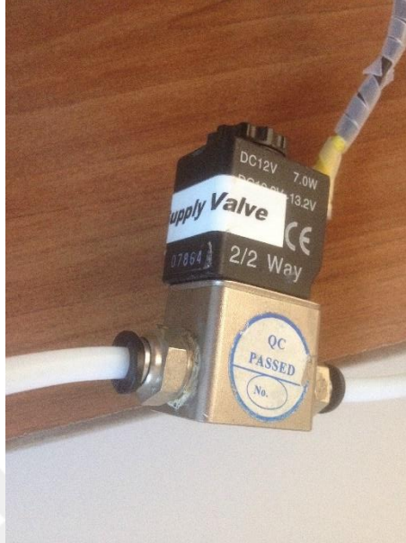
Figure 3.4. Hydrogen supply valve
