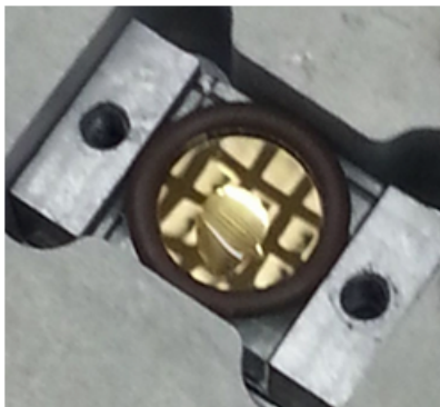
Figure 5.12: Photo of the sample holder of the device after an experiment. The fluid channel is filled with water during the removal of the PTFE channel.
