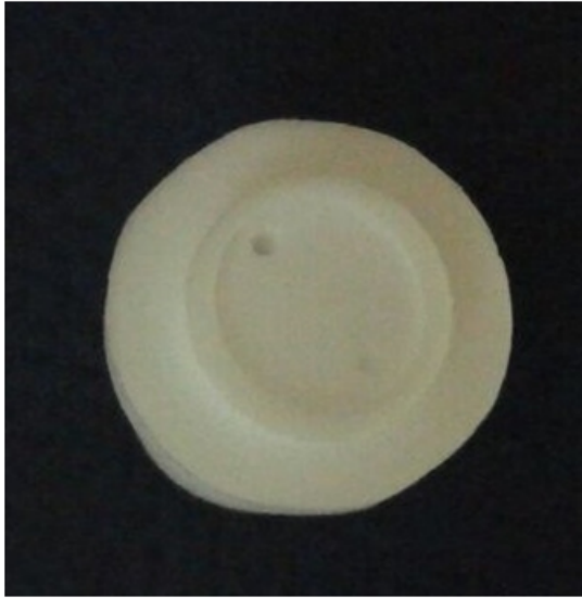
Figure 5.11: Modified PTFE channel is shown. In this channel design, the interaction of fluid with o-ring is prohibited.
