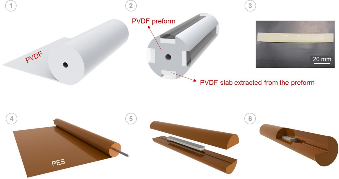
Figure 3.4: The fabrication steps of the PVDF ribbon embedded in PES preform which is a macroscopic copy of the final nanoribbons. As an initial step, (1) a PVDF preform is built by rolling PVDF sheets and (2-3) a slab is mechanically extracted out of the PVDF preform. (4-5) Next, the PVDF slab is inserted into a PES preform which is then sealed by heating in a consolidator oven. (6) The final multimaterial product turns into a PVDF ribbon embedded PES matrix. Dimensions and design specifications of the preform directly affect the size and shape of the final product of the drawing process.
