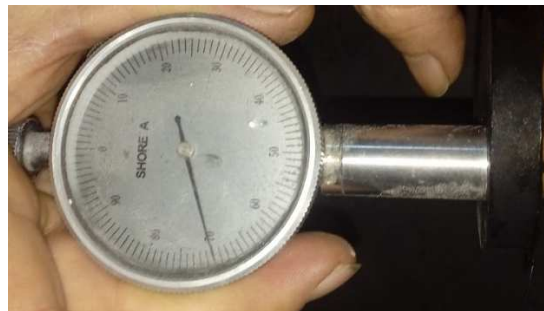
Figure 4.12 Testing the manufactured rubber sample hardness (Personal archive, 2019)
