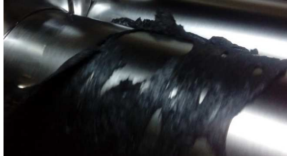
Figure 4.5 Sticky Congolese rubber mixed with Vietnamese rubber on the roll-mill (Personal archive, 2019)
