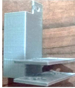
Figure 3.37 Solenoid housing 3D print (Personal archive, 2019)
