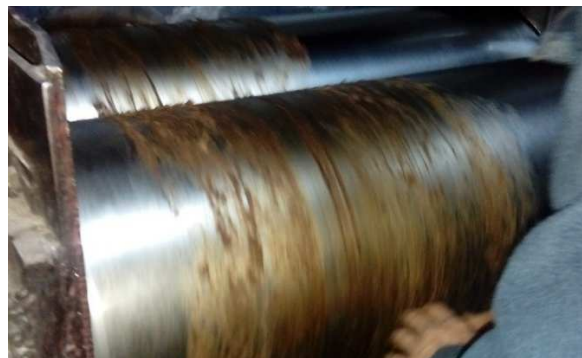
Figure 4.4 Sticky Congolese rubber on the roll-mill (Personal archive, 2019)
