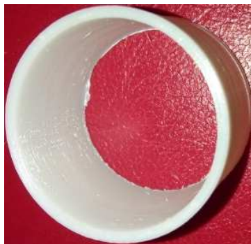
Figure 3.33 Dust filter 3D print (Personal archive, 2019)
