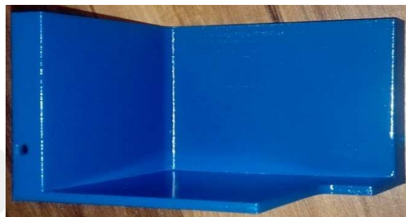
Figure 3.35 Back cover-Electronic box A 3D print painted (Personal archive, 2019)
