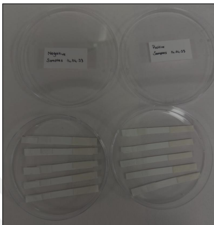
Figure 3.8.3 Examples of positive and negative strip designs
