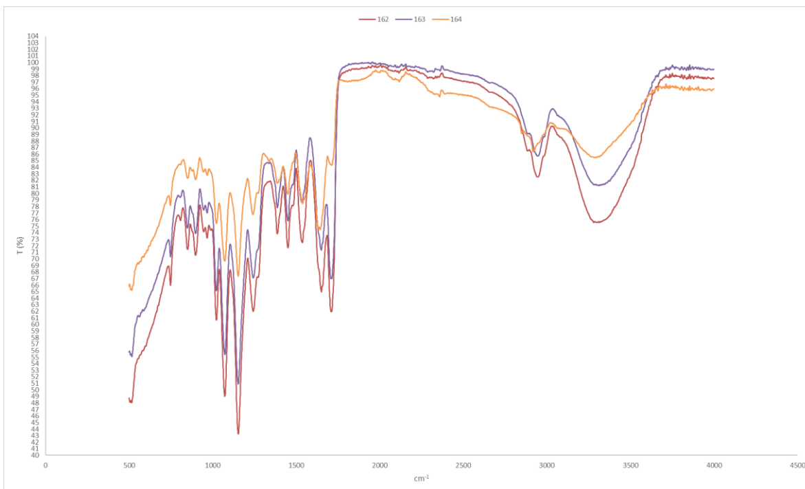
Figure 4.2. The FTIR spectra of cryogels coded as 162, 163 and 164.
