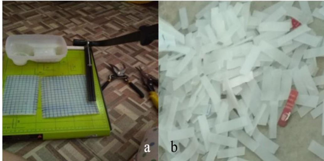
Figure 2.15 The preparation of high-density polyethylene (HDPE) plastic fibers, including (a) the preparation for the cutting process and instruments, and (b) HDPE 192 fibers with a size of 0.5 x 2 cm (Rahman and Nurdiana 2020)
