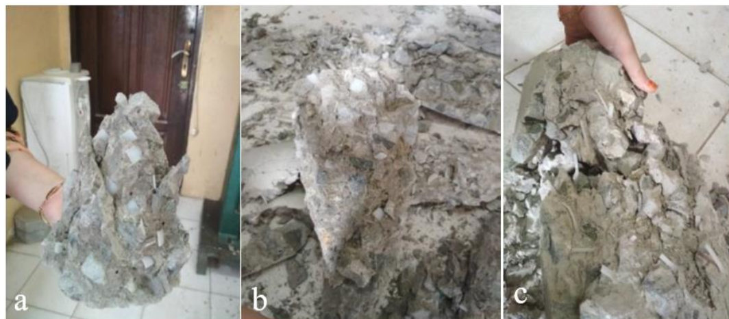
Figure 2.16 Visualization of the state of the HDPE fibers: (a) 1 centimeter by 1 centimeter, (b) 0.5 centimeters by 2 centimeters, and (c) 0.25 centimeters by 4 centimeters (Rahman and Nurdiana 2020)
