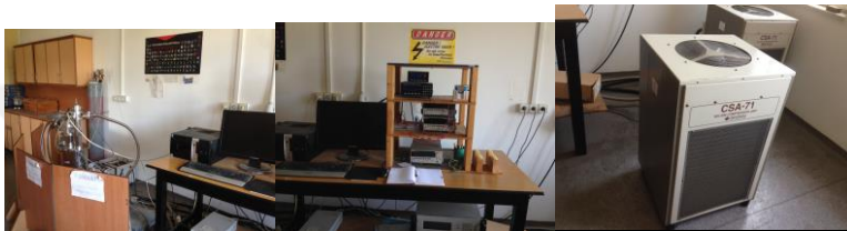
Picture 3. 4: Cyclic cryogenic refrigeration system.
