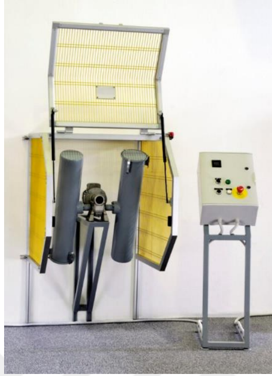
Şekil 4.9. CSR (Coke Strength after Reaction) tamburu [30]
