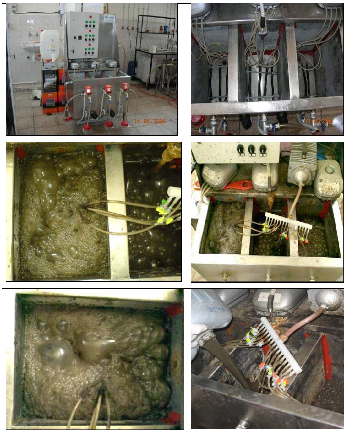
Figure 4.1. Aerobic tanks used in this study and some pictures from the reactor operations
