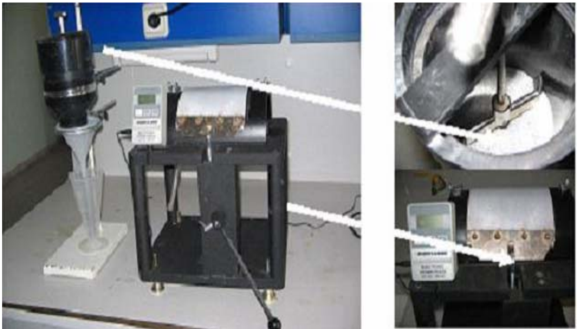
Figure 4.10. Gravity drainage plow simulator kit and Crown press used in this study (Ayol et al. 2007)
