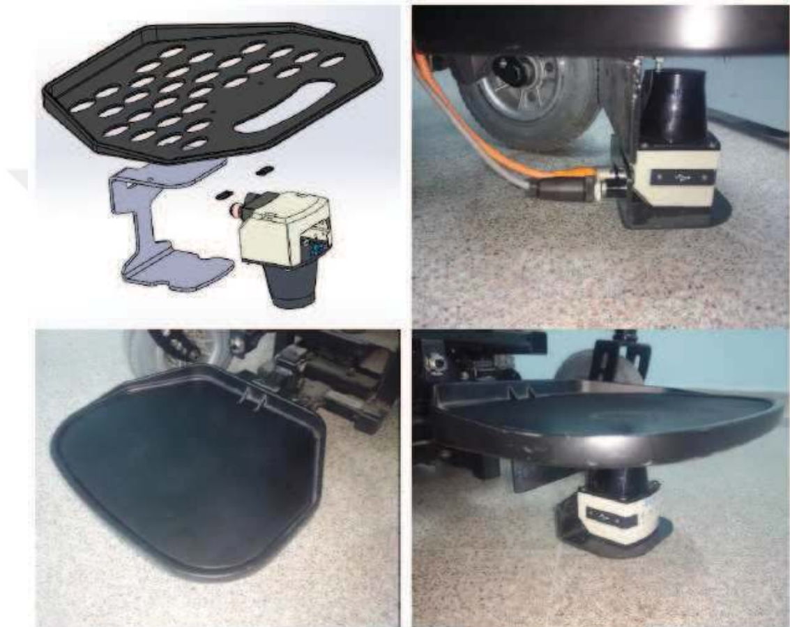
Figure 3.10 Protection cage of LIDAR under legroom of the wheelchair for the second prototype
