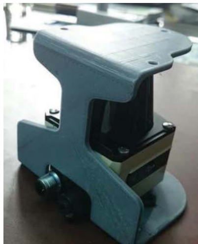
Figure 3.9 Protection cage of LIDAR produced by 3D printer (Personal archive, 2015)
