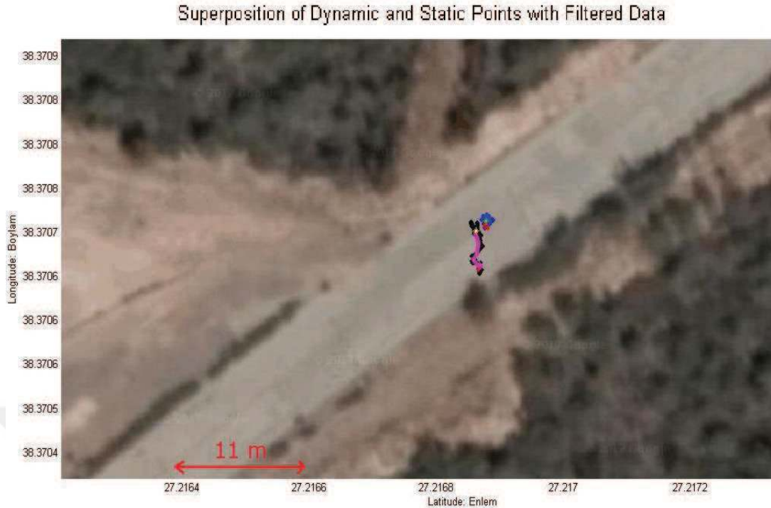
Figure 2.22 Superposition of raw (blue and black) and filtered (purple and red) GPS position data
