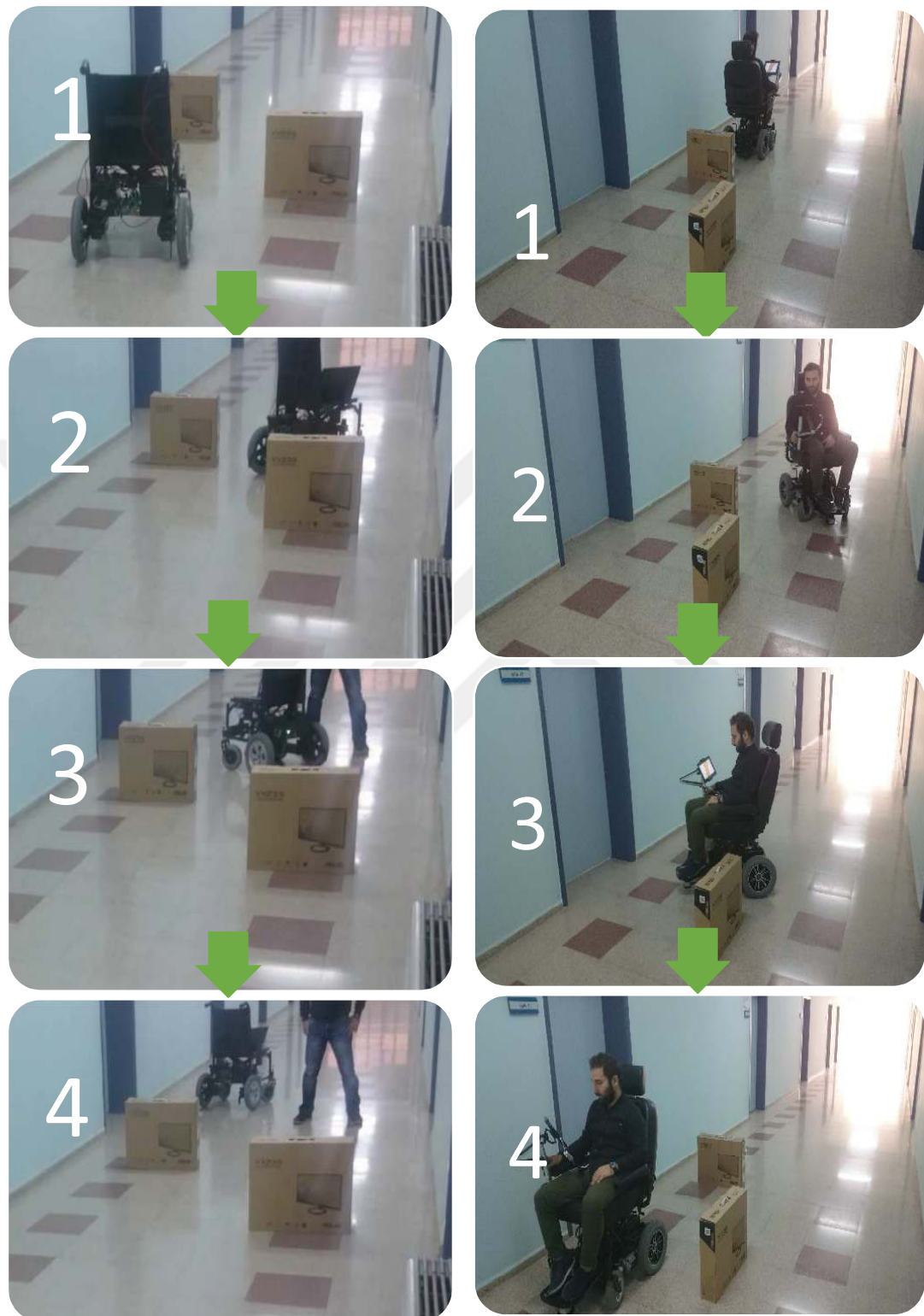
Figure 7.16 Real-time autonomous driving tests with static and dynamic obstacles (Personal archive, 2016)
