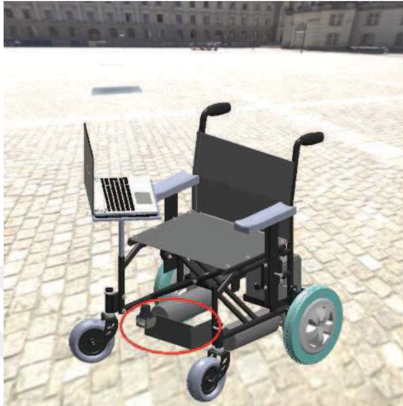
Figure 3.8 Final design of the vehicle with LIDAR
