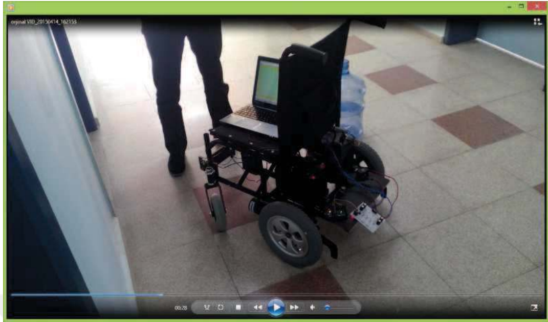
Figure 7.13 Real-time autonomous driving tests with dynamic obstacles (Personal archive, 2016)
