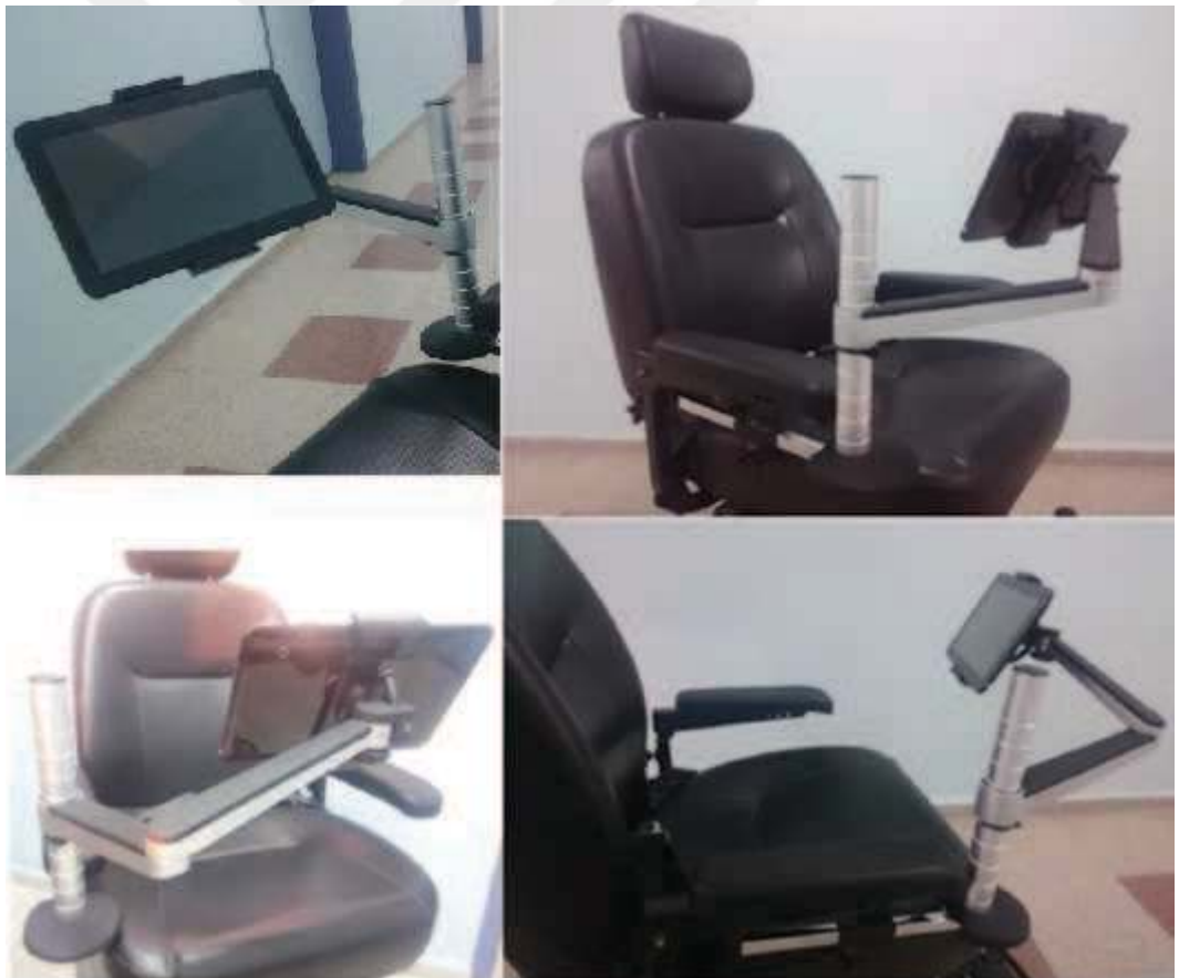
Figure 3.5 Implementation of the functional tablet/monitor holder (Personal archive, 2016)
