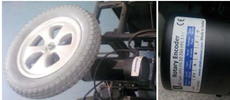
Figure 2.14 Encoder directly connected to motors for the first prototype (Personal archive, 2014)
