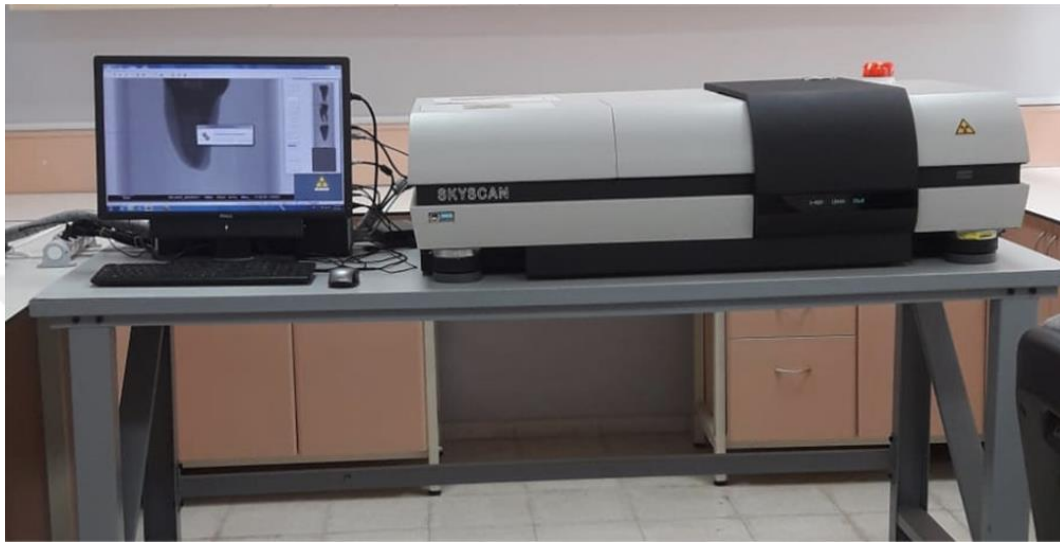
Figure 14: First Micro Ct scanning of all samples were performed with Bruker-Micro-CT device.
