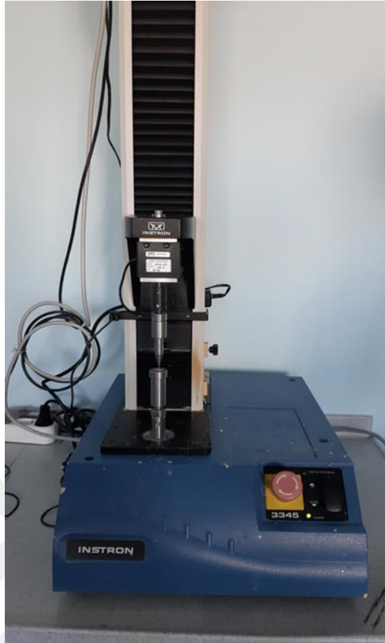
Figure 18e: Universal Testing Machine, Instron (Lloyd LRX; Lloyd Instruments Ltd, Fareham, UK); that used in push out testing in order to calculate bond strength of samples.
