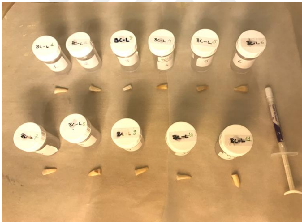
Figure 7a: Group BC-L: Samples in this group were obturated with TotalFill BC Sealer and Lateral Condensation.
