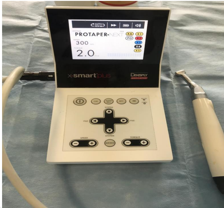
Figure 3c: Endodontic motor Dentsply x-smart plus (Dentsply Maillefer, North America) adjusted to: 300rpm speed, 2.0 torque for chemo-mechanical preparation of the samples.
