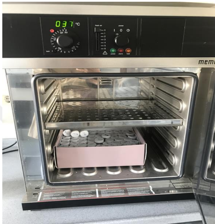
Figure 13: After obturation of the samples were completed, all samples were stored in 37 degrees 100% humidity for 7 days.
