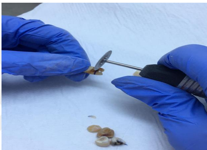
Figure 2a: Separation of crowns from sample teeth.
