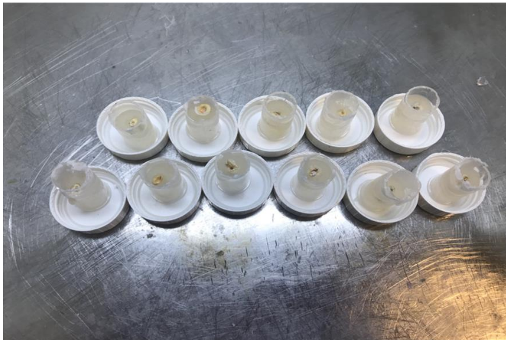
Figure 18b: Samples were fixed with acrylic inside plastic tubes.
