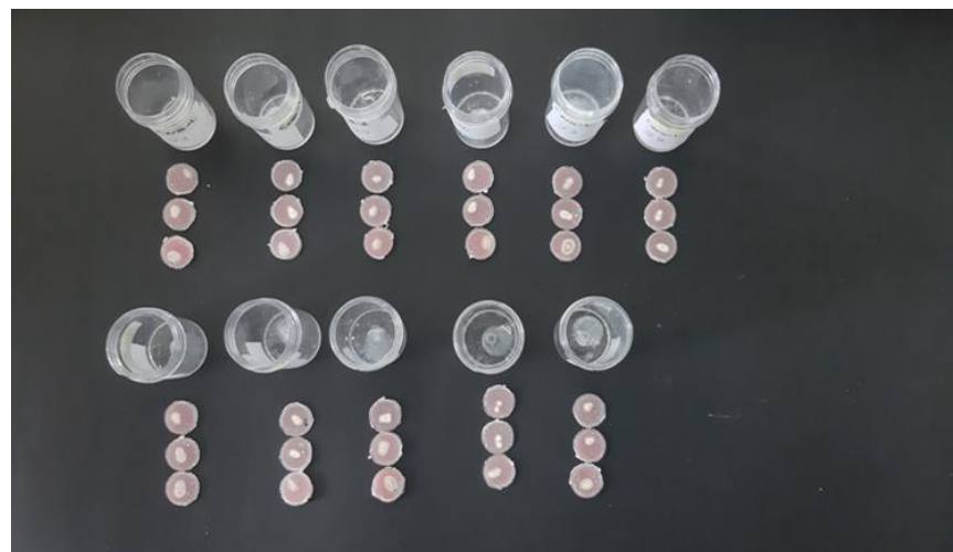
Figure 19b: 1mm thick dentin discs were prepared from the samples of Group (BC-S)
