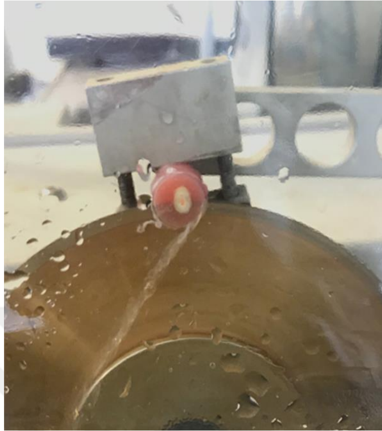
Figure 18c: 1mm thick dentine discs were obtained with the help of Isomet device.
