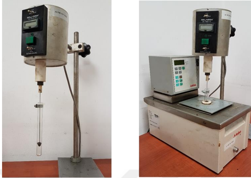
Figure 3.4 Outlines of gelation instrument and thermoregulated oil bath device
