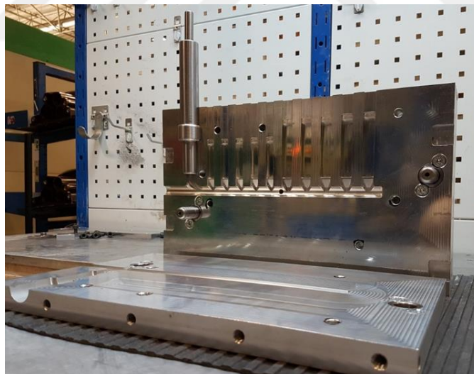
Figure 3.11 Machined aluminium mold in open position showing the cavity of SENB test specimens
