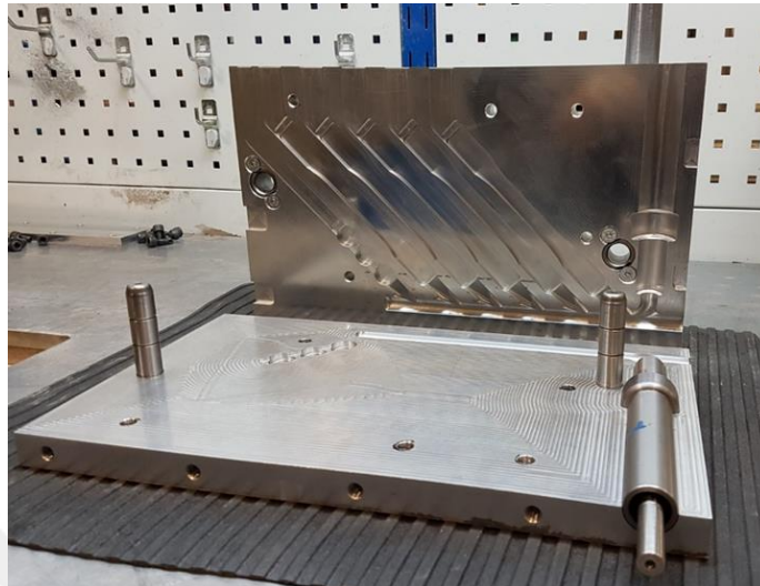
Figure 3.10 Machined aluminium mold in open position showing the cavity of tensile test specimens
