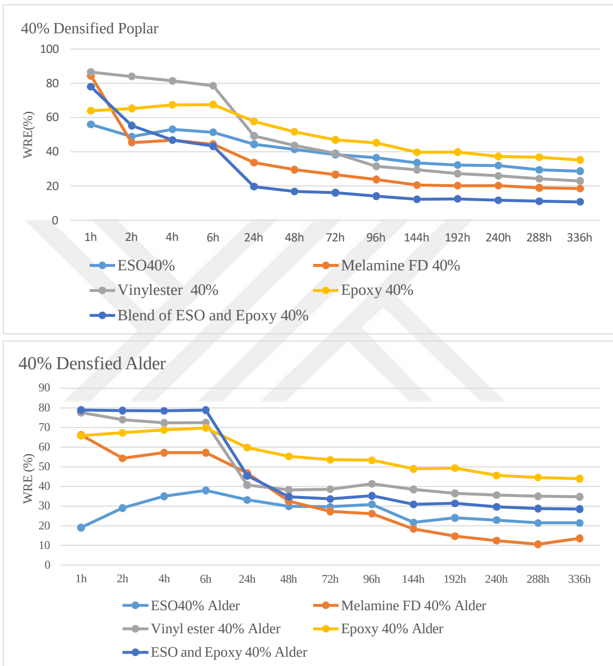
Figure 8. Water repellence efficiency of 40% compressed poplar (upper) and Alder wood (lower)
