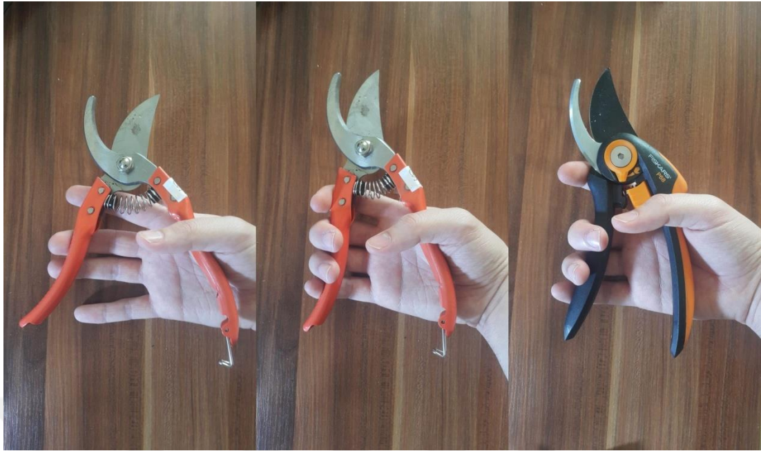
Figure 6.5 Full open positions of the pruning shears (left and right), holding position with the little finger (middle) (Personal archive, 2019)
