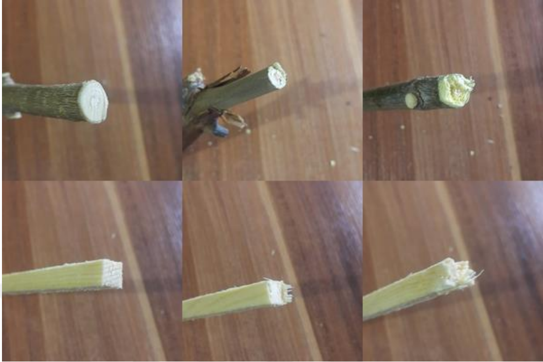
Figure 6.11 Good cutting surface (top left-live bough), normal cutting surface (top middle-live bough), bad cutting surface (top right-live bough), good cutting surface (bottom left-7mm pine bough), normal cutting surface (bottom middle-7mm pine bough), and bad cutting surface (bottom right-7mm pine bough) (Personal archive, 2019)
