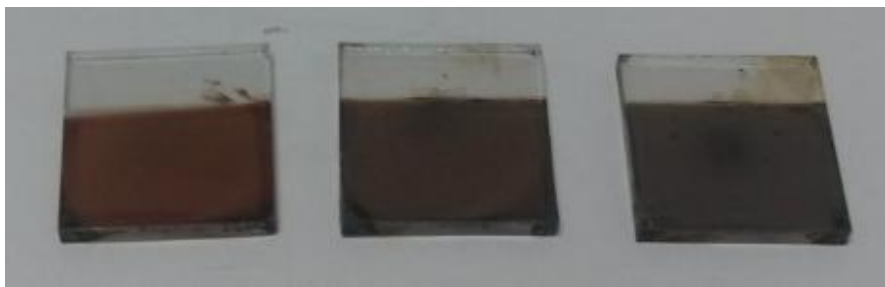
Figure 48. Photographs of the 6-Cd(II)/surfactants mole ratio samples loaded , 2 and 3 times reacted under H_2Se (left to right).
