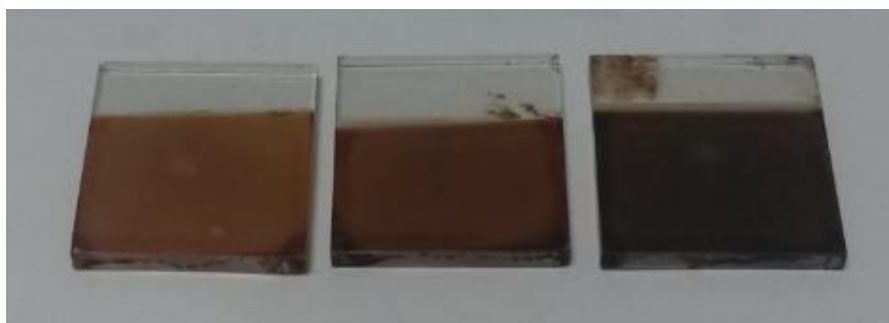
Figure 46. Photographs of the 4, 6, and 8-Cd(II)/surfactants mole ratio samples loaded once and reacted with H_2Se (left to right).
