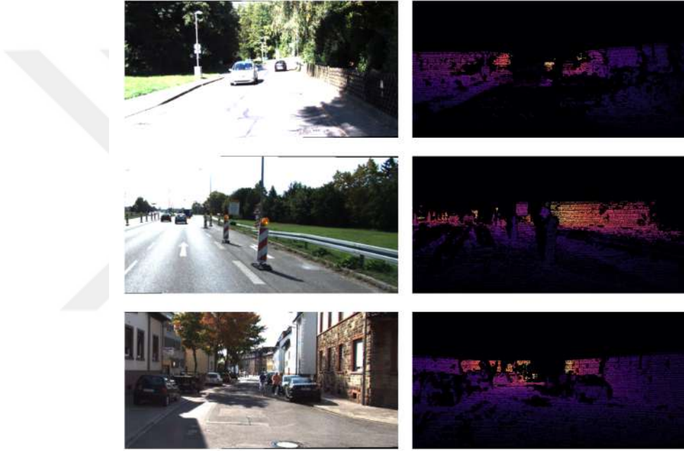
Figure 34: The depth maps from LIDAR visualised as normalized heat-maps on right and matching RGB images on left. Samples are selected from KITTI training dataset
