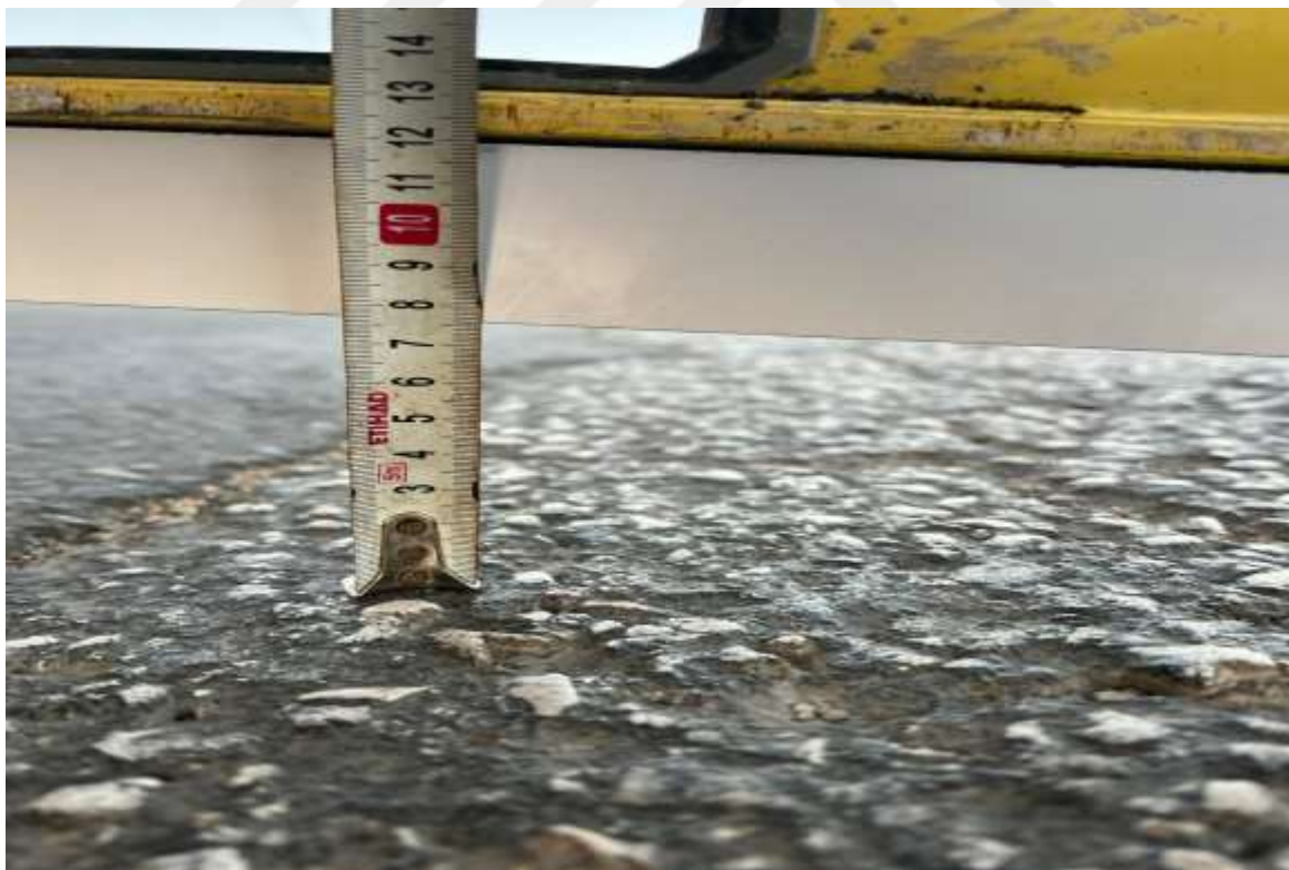
Figure 3.5: Sample Of Measuring Rut's Length Manual Method Using Meter and Ruler.
