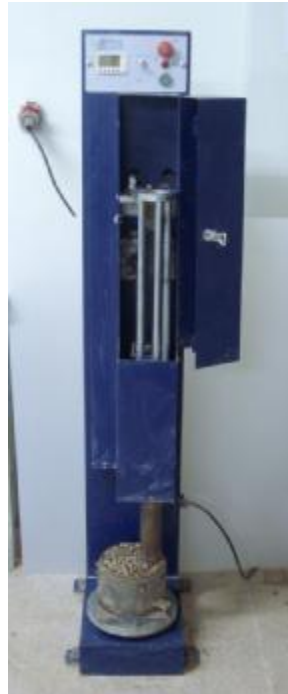
Figure 4.4 Automatic soil compactor machine
