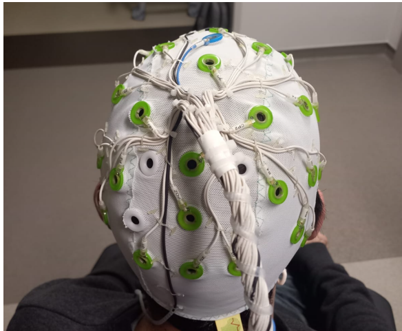
Figure 3.3: MR Compatible 32 Channel EEG Cap (Brain Products) used in our study.
