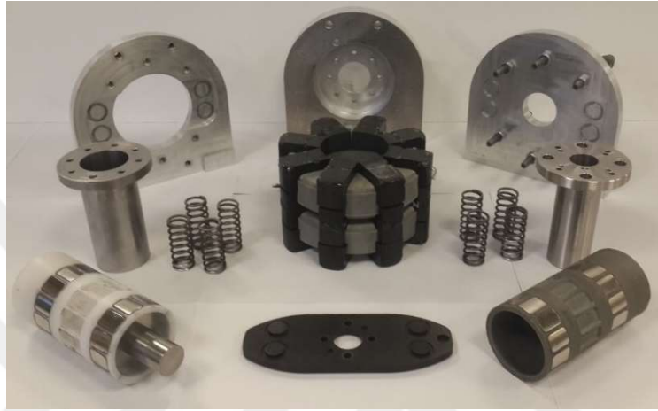
Figure 7.14: Disassembled view of the manufactured parts of the moving magnet linear actuator
