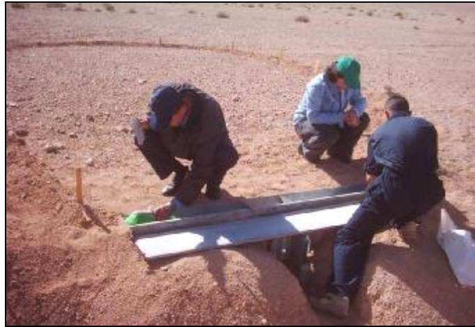
Figure 3.15. Gerlach Trough for Soil Loss Measurement at Micro-catchment Scale.
