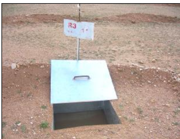
Photo 12. A Tank with Runoff and Sediment after a Runoff Event
