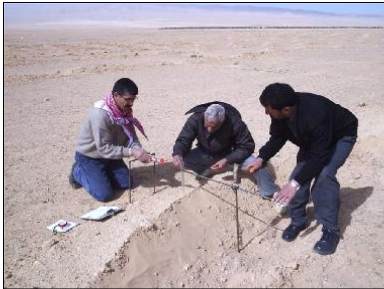
Figure 3.19. Bridge Frame for Ridge-decay Measurement
