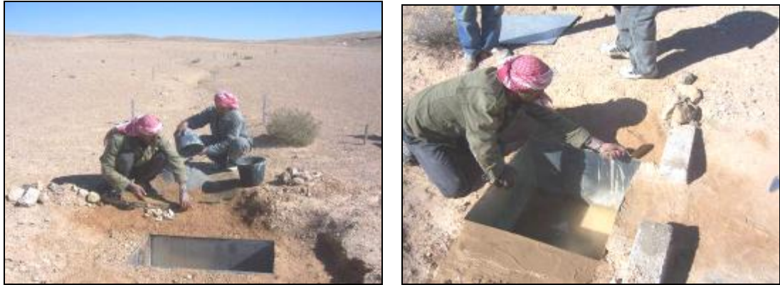
Figure 3.17. Catch-trap for Measurement of Sediment Yield at Rills Scale
