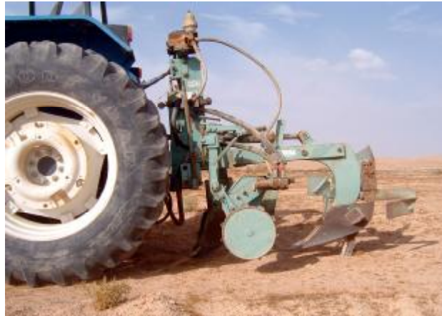
Photo 19. Vallerani Implement that can Develop Continuous and Intermittent Ridges
