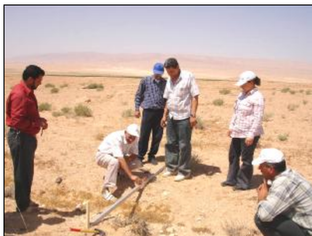
Photo 9. Installation of Bridge Frames for Rill Measurement were checked for Horizontal and Vertical Controls
