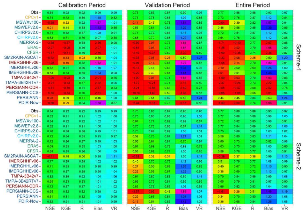
Figure 3.40. Performance of daily streamflow simulations at the Karasu basin outlet using the gauge and 18 GPDs data considering calibration, validation, and entire period. Y-axis color presents: satellite-based (blue), gauge and satellite (red), reanalysis and satellite (sky blue), reanalysis (green), reanalysis, ground, and satellite (steel blue), and ground (yellow).
