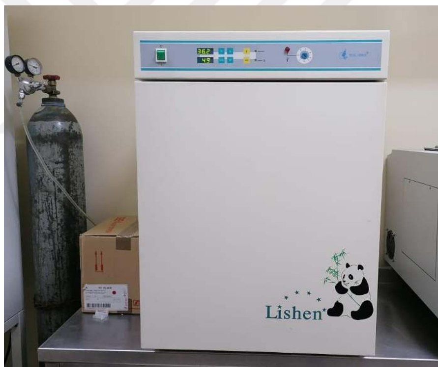
Figure 3.10. CO 2 incubator used to keep atmosphere of the medium and culture of the cells
