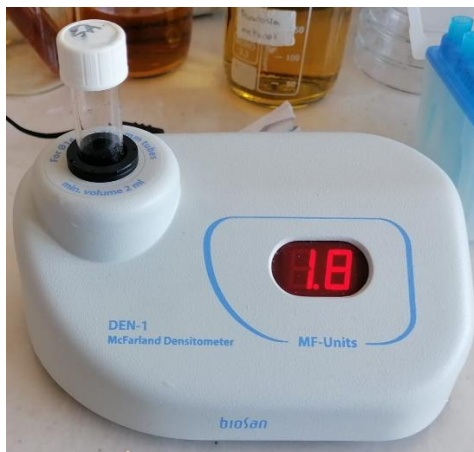
Figure 3.4. DEN-1, McFarland Densitometers instrument that used for the measurement concentration of both bacterial and yeast cells (during the antimicrobial activity used)
