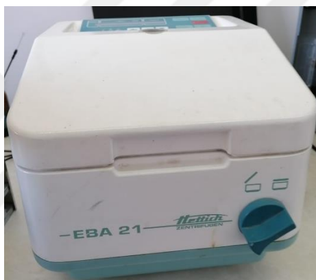
Figure 3.5. Centrifuge instrument that used for separating particles from a solution by applying centrifugal force
