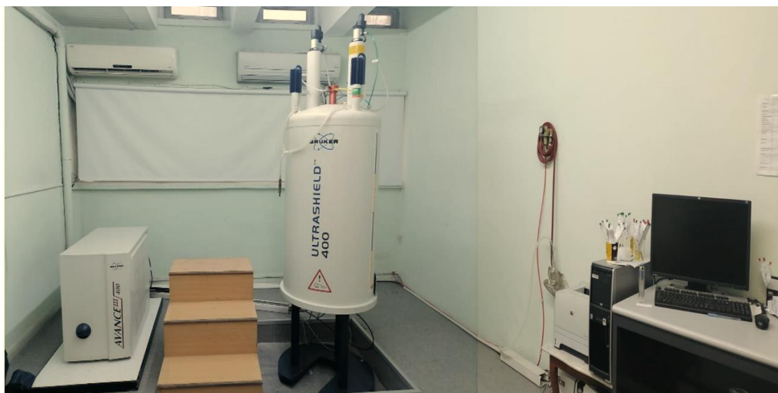
Figure 3.7. NMR instrument that used to identify the chemical structure of the compound
