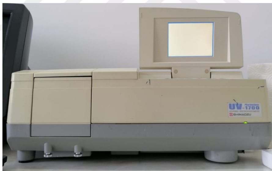
Figure 3.3. UV-visible spectrophotometry instrument that used for evaluation AOA at various absorbance
