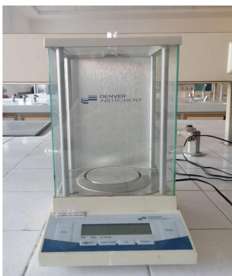
Figure 3.6. A sensitive balance instrument that used to weigh numerous compounds with extremely accuracy
