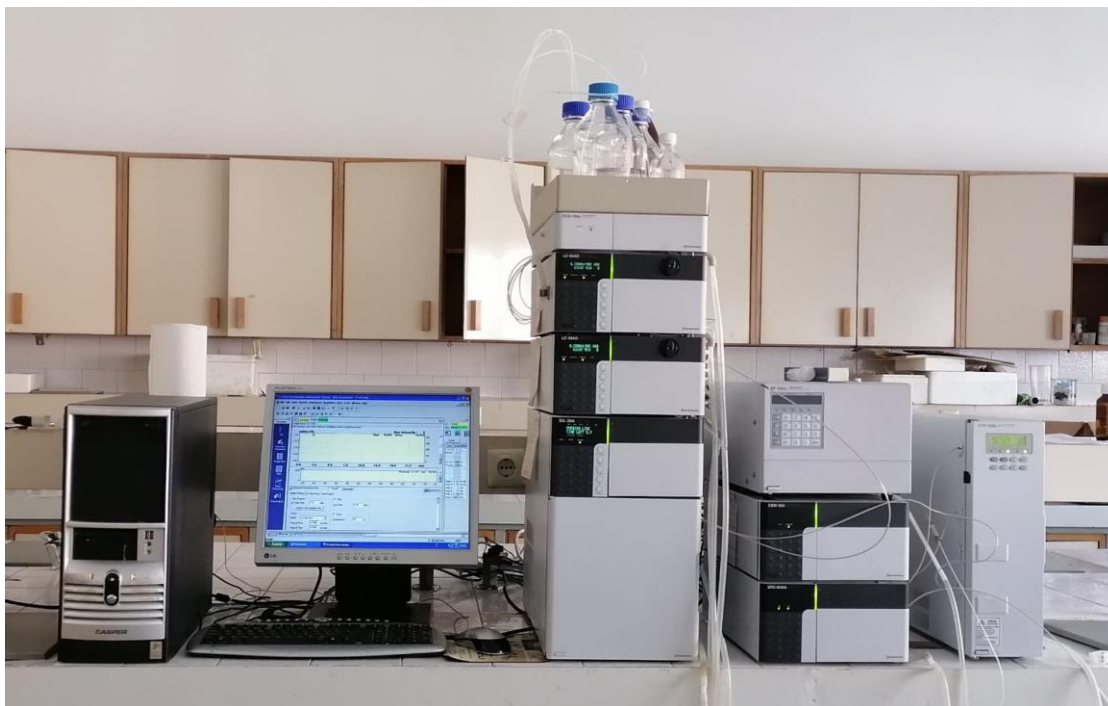
Figure 3.2. HPLC instrument that used for investigation vitamin A, C, E respectively at 326nm, 254nm, 296nm
