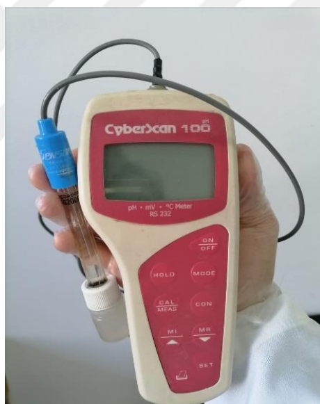
Figure 3.1. A pH meter instrument that used for measurement concentration hydrogen-ion in a particular solution to achieve its pH value (during AOA used)
