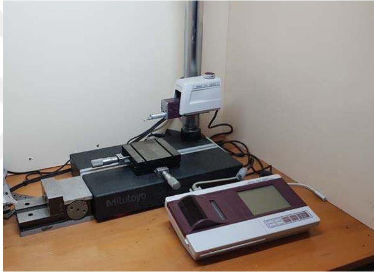
Figure 4.8. Profilometer used to evaluate surface roughness of the blanks
