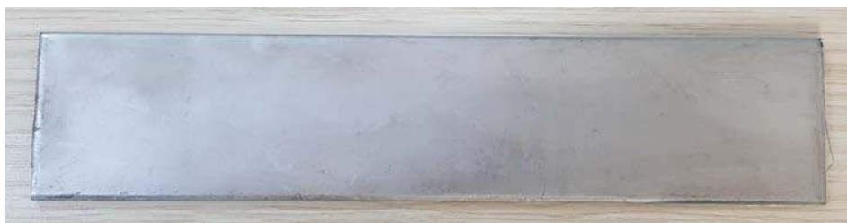
Figure 4.7. AISI 304 sheet metal specimen used for blanking experiments (t= 2 mm)
