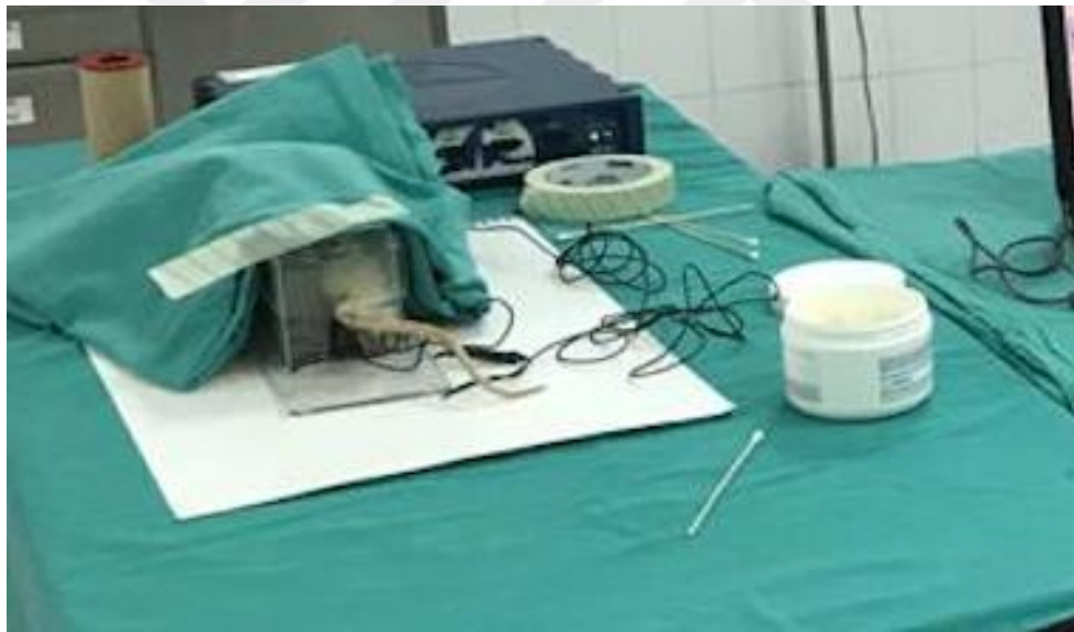
Figure 3. 2 The immobilizer, electrode paste and electrodermal electrodes of EDA
