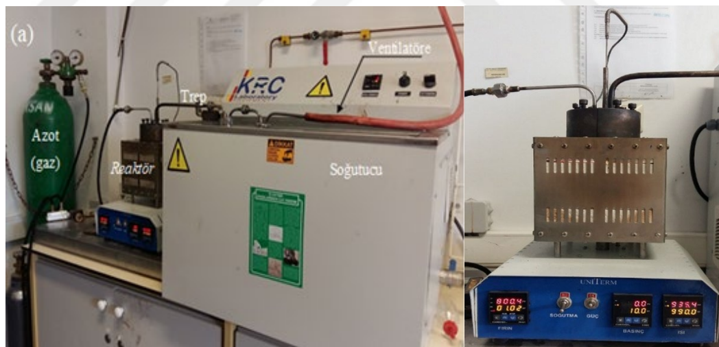
Figure 7.4. (a) Experimental setup for carbonization , (b) Carbonization Reactor .
