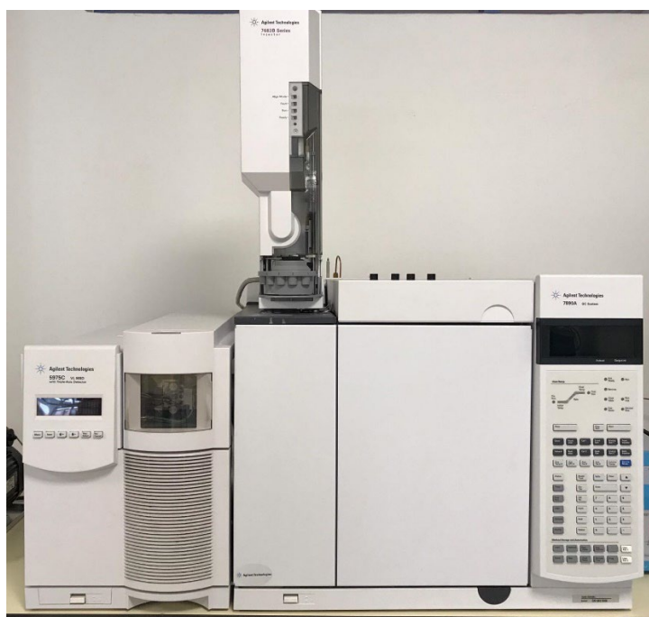
Figure 7.6. GC-MS for Oil Analysis
