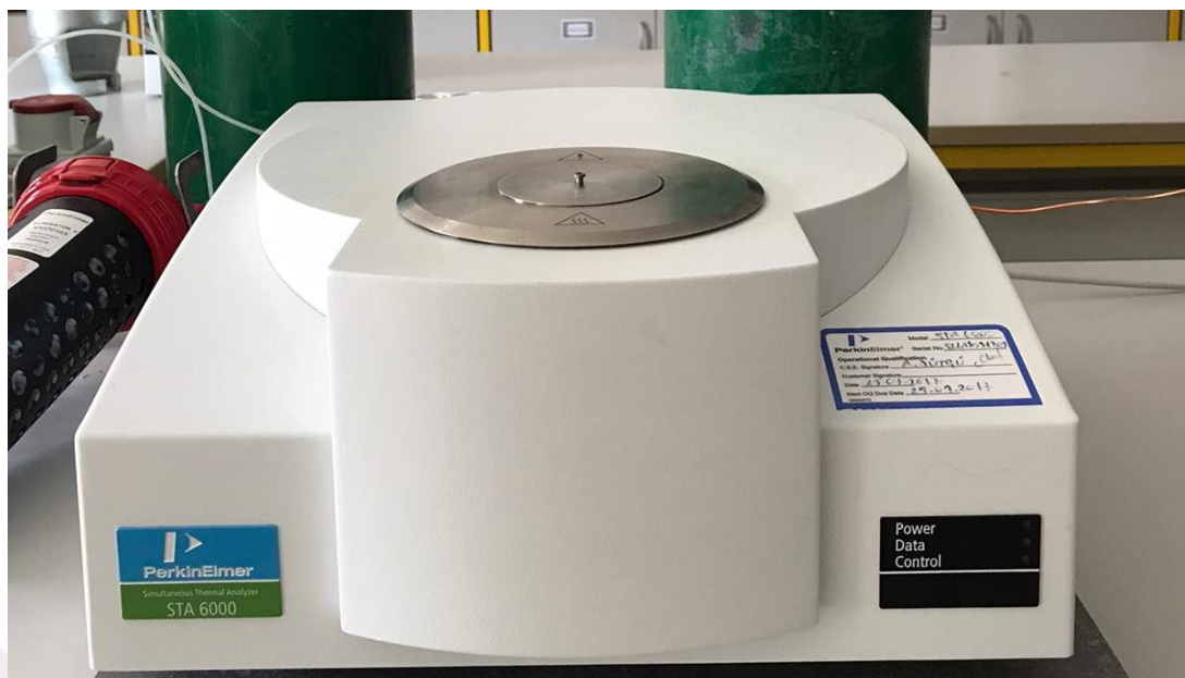
Figure 7.2. Thermogravimetric analyzer (Perkin Elmer Simultaneous Thermal Analyzer, STA 6000)
