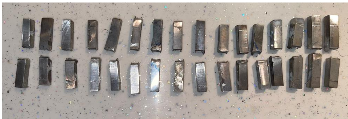
Figure 4.3. Notch Impact Test Samples After Tests
