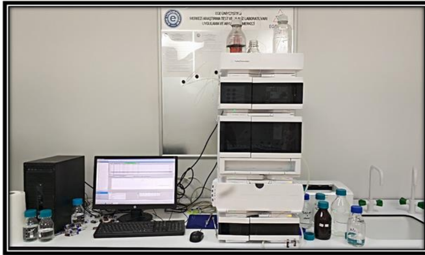
Resim 6. Agilent 1260 Infinity II Quaternary LC HPLC cihazı
