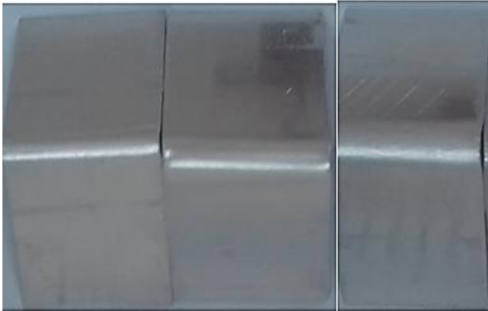
Figure 3.6a: Bend Specimen Viewed under x30 Magnification: Exterior
