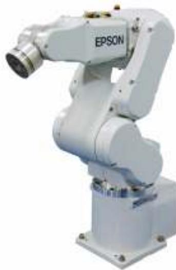
Figure 2.3 Articulated robot (C3 Series, Epson)
