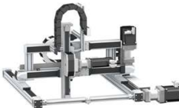
Figure 2.4 Cartesian robot (Lexium MAX, Schneider Electric)
