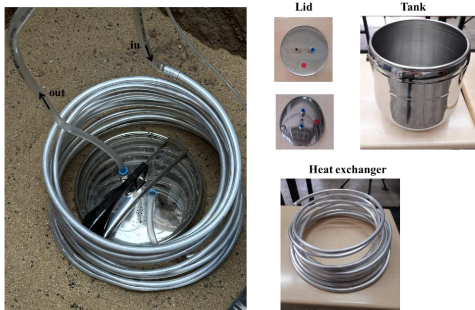
Figure 7.23. Underground metal tank and aluminum heat exchanger
