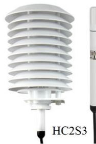
Figure 7.7. The air temperature and humidity sensor
