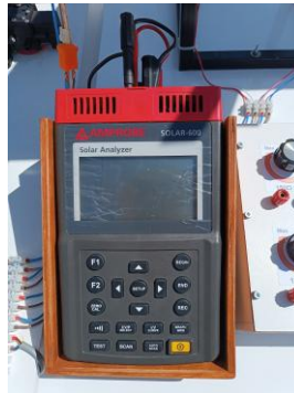
Figure 7.9. Solar power analyzer
