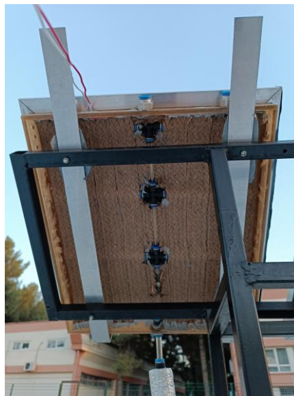
Figure 7.28. Test setup of the cooled panel
