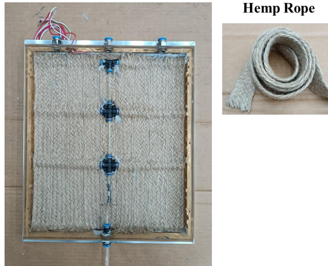
Figure 7.27. Cooled PV Panel with attached hemp rope.
