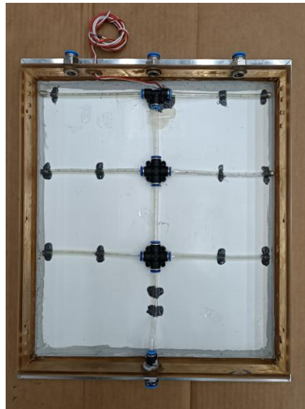
Figure 7.20. The liquid distribution system on the rear side of the panel
