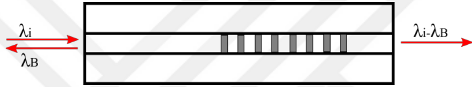
Figure 3.3: An exemplary FBG that reflects part of wavelength that satisfies Bragg condition.
