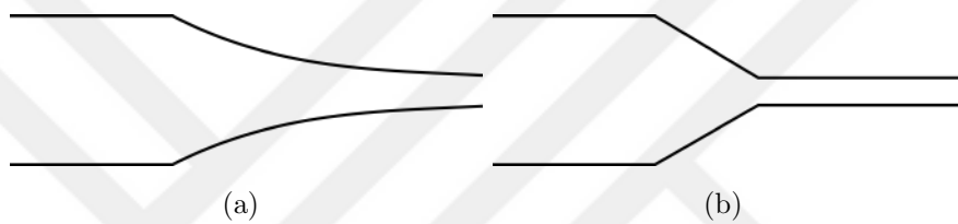
Figure 3.12: Variation of taper angle for both: (a) adiabatic taper, (b) non adiabatic taper .
