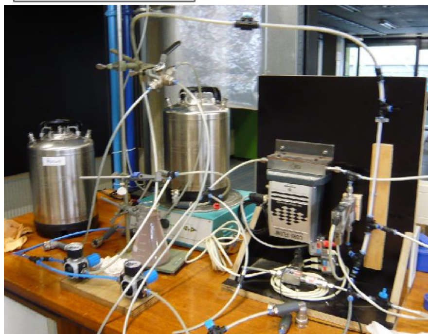
Figure 3.3 : Schematic diagram of the SUR measurement experimental setup (A: demineralized water vessel; B: wastewater vessel; C: magnetic stirrer; D: three-way valve; E, H, I, K: valves; F: flow meter; G: membrane module; J: computer with measuring program; L: permeate vessel; P: pressure difference sensor).
