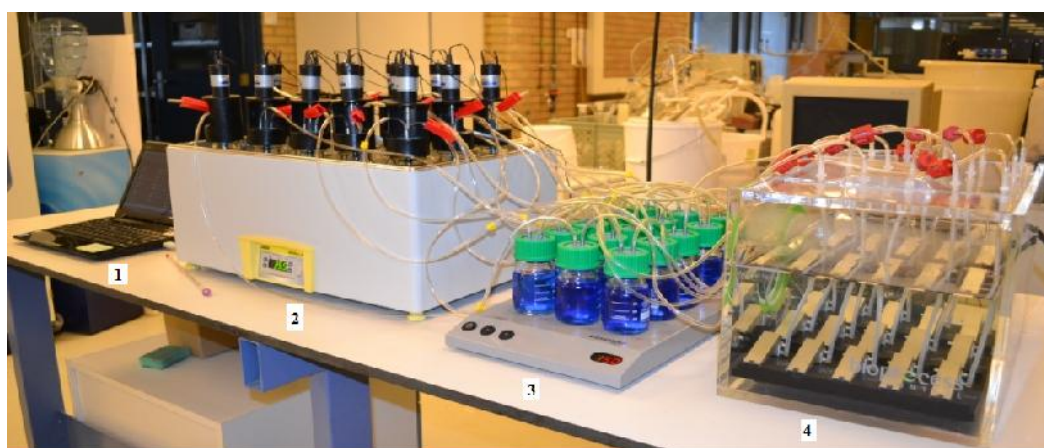
Figure 4.2 : AMPTSII (1- Data storing, 2- Glass reactors with mixing and water bath, 3- CO 2 fixation unit, 4- Flow cell with methane production).
