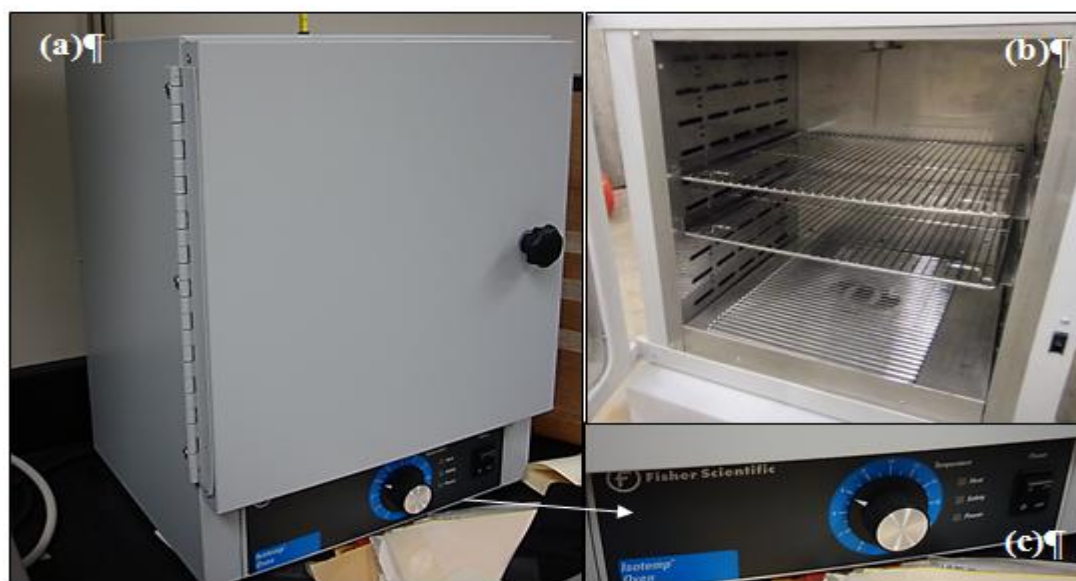
Figure 4.13. a) Fisher Scientific™ Isotemp™ Oven b) Inside of the Fisher Scientific™ Isotemp™ Oven and c) Control Panel of Fisher Scientific™ Isotemp™ Oven.
