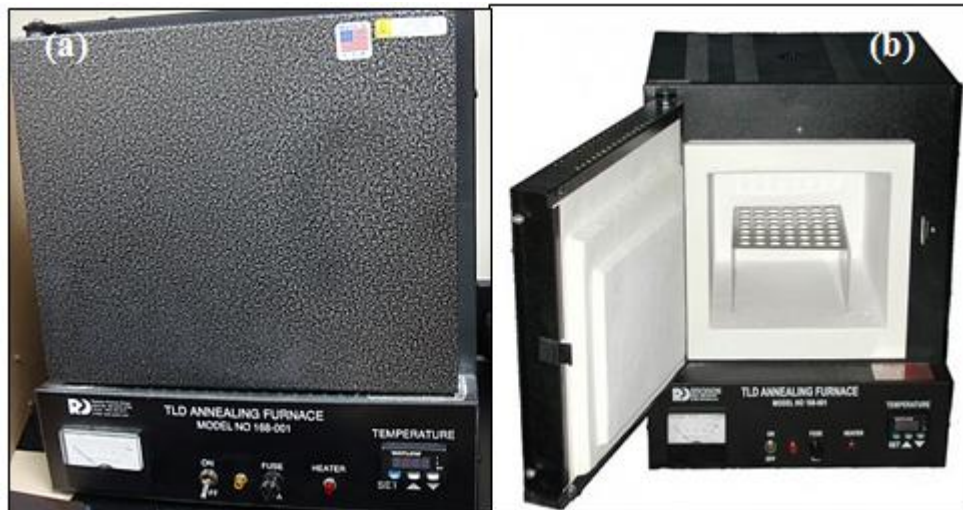
Figure 4.14. a) TLD Annealing Furnace 168, 001 (120 VAC) Radiation Product Design. b) Inside of the TLD Annealing Furnace 168, 001.
