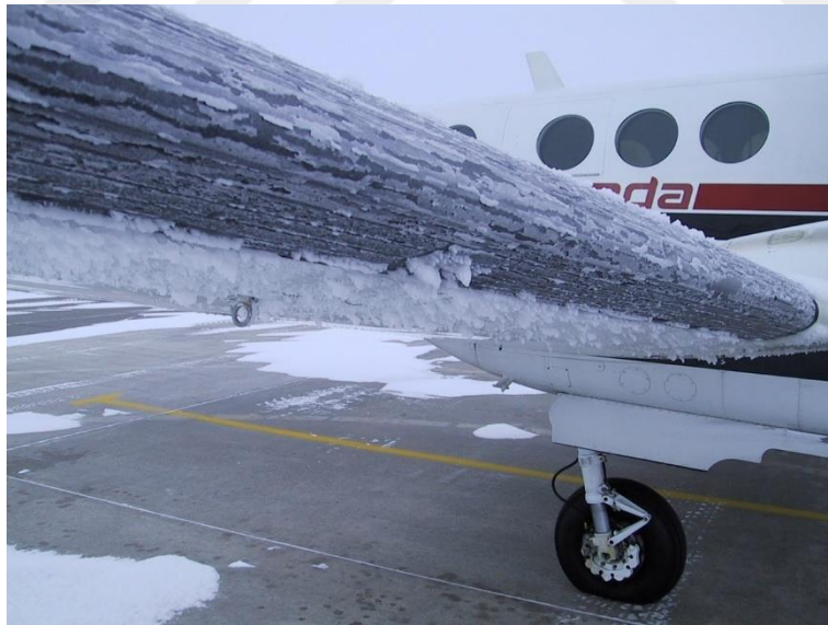
Figure 1.1: Ice accretion on an aircraft wing [1]
