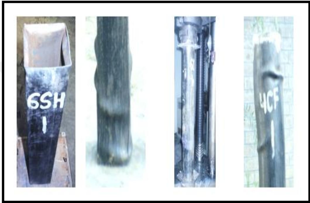
Figure 2.8 Photographs showing failure modes of columns (Kibriya, 2006)
