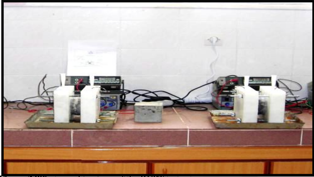
Figure 3.8 Photographic views of the RCPT test setup
