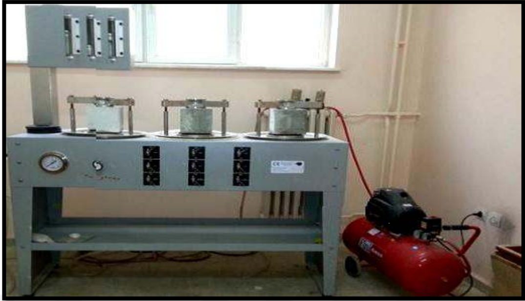
Figure 3.7 Measurement of water permeability test setup
