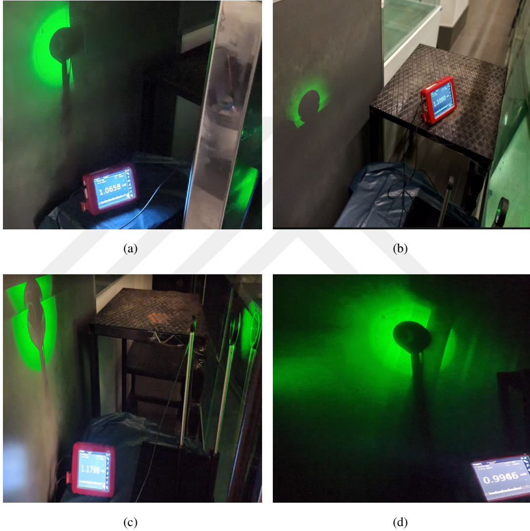
Figure 30: Reflection measurements from different orientations of a reflector at (a) right side (b) bottom (c) top and (d) diagonal.
