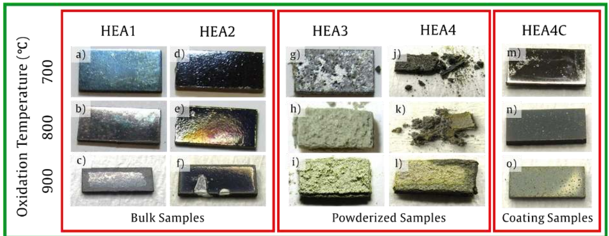
Figure 2.1. Photographs showing the state of the samples following the oxidation experiments
