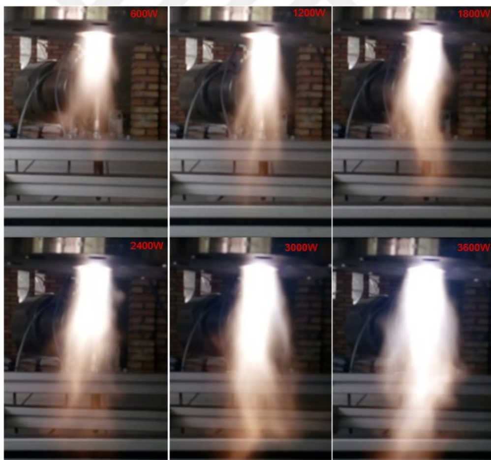
Figure 3.20 Effects of microwave power on plasma flame in case 50 sL/min air flow rate
