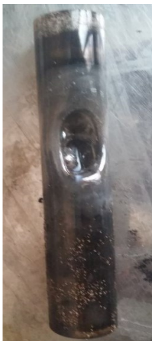
Figure 3.28 Deformed quartz glass because of low air flow rate input and moisture content of fuel
