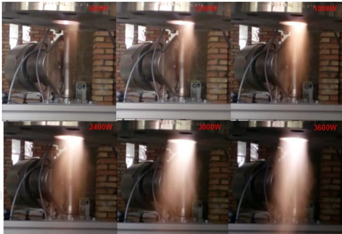
Figure 3.23 Effects of microwave power on plasma flame in case of 27 L/min water steam and 50 sL/min air flow rate
