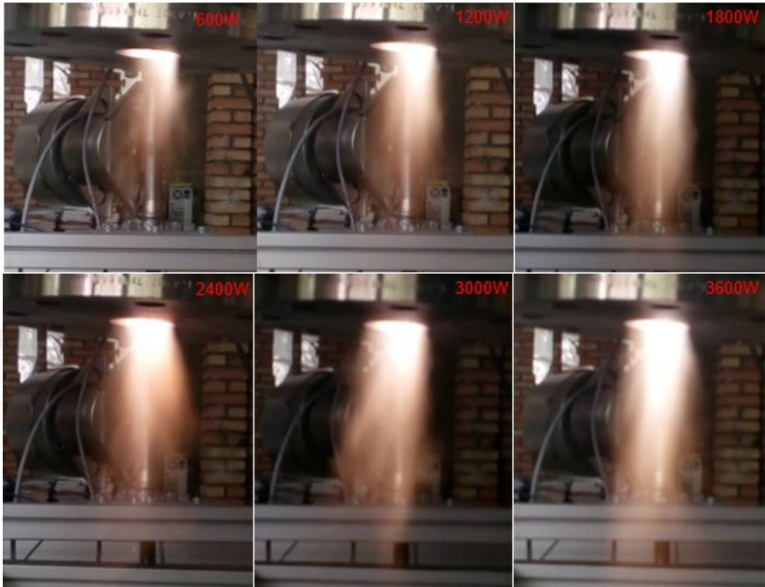
Figure 3.22 Effects of microwave power on plasma flame in case of 18 L/min water steam and 50 s L/min air flow rate
