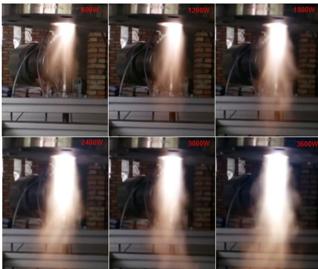
Figure 3.21 Effects of microwave power on plasma flame in case of 9 L/min water steam and 50 sL/min air flow rate
