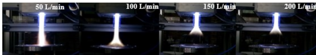
Figure 3.19 Effects of the air flow rate on plasma performance in case of 3600W plasma power
