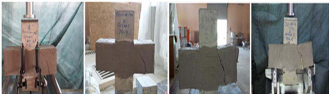
Figure 4.7 The mode of failure in the Basalt Fiber Mesh (Rupture in the Fibers)
