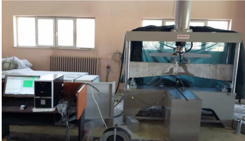
Figure 3.4 Test setup for four-point loading test
