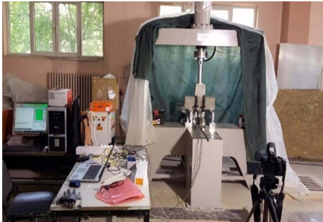
Figure 4.5 Corbel Setup on the test machine
