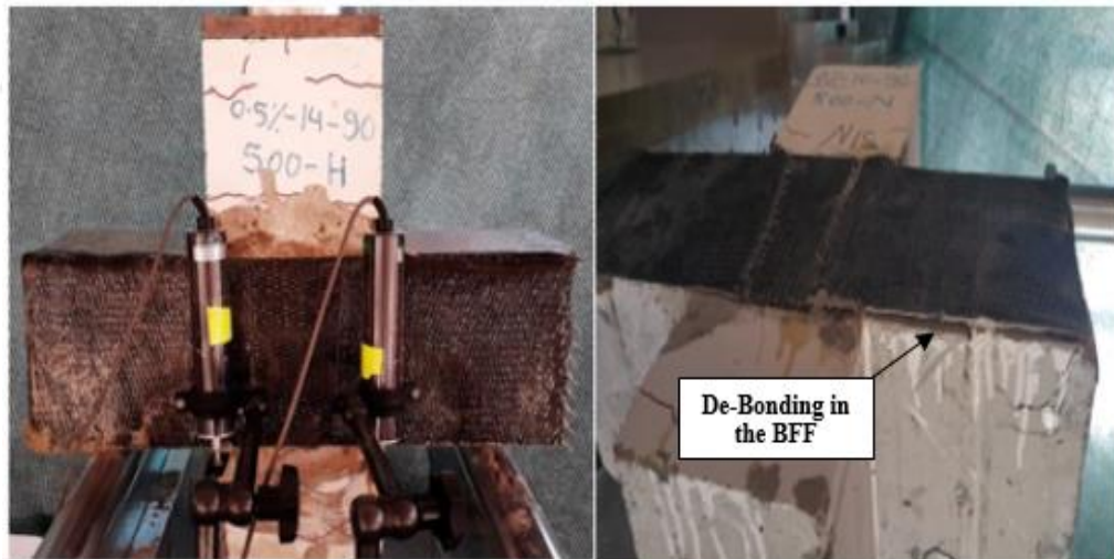
Figure 4.12 BFF-strengthened specimen with de-bonding failure
