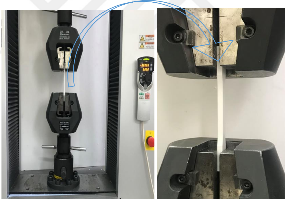
Figure 3.7 Sample geometry for tensile test of FDM printed parts [56]
