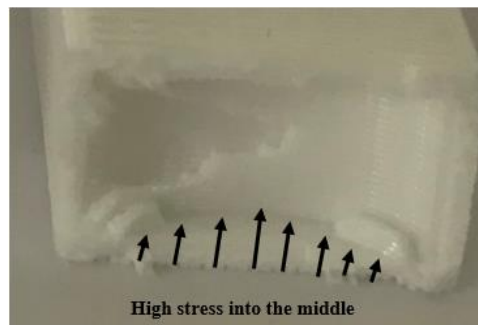
Figure 4.12 Section of Archimedes pattern with 60% infill ratio
