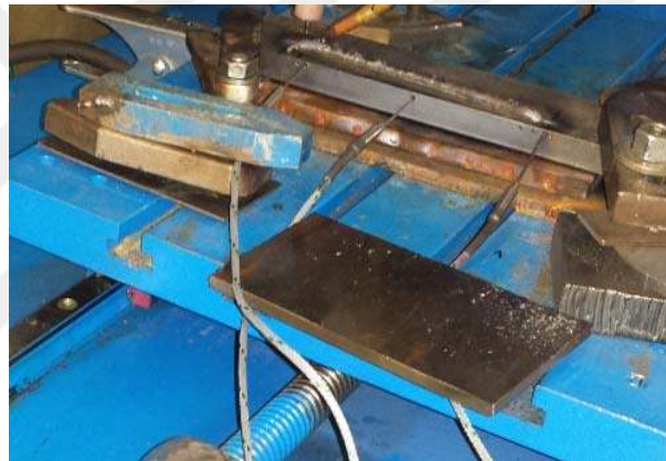
Figure C.1. (a) general view of the data logger with 3 K-type thermocouples; (b) the details of the screen displays (c) attaching the thermocouples in the located positions
