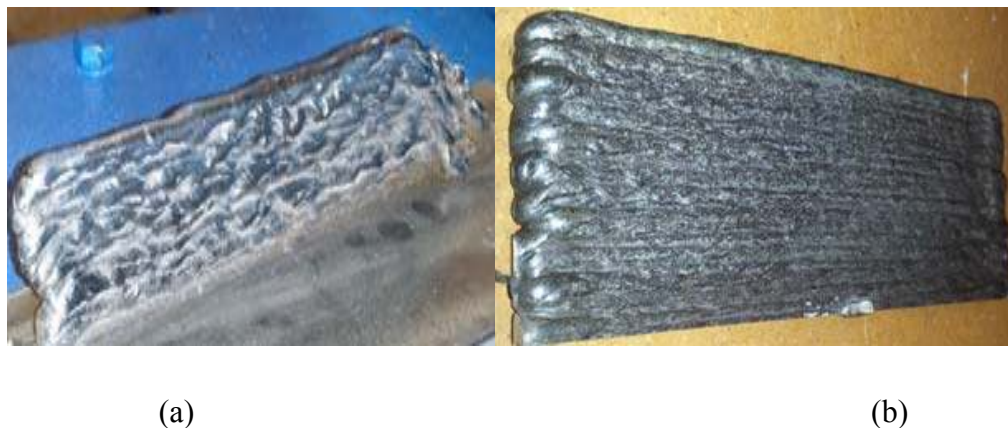
Figure 4. 97. Photographs illustrate deposited walls using (a) one direction during deposition and (b) reverse direction deposition method
