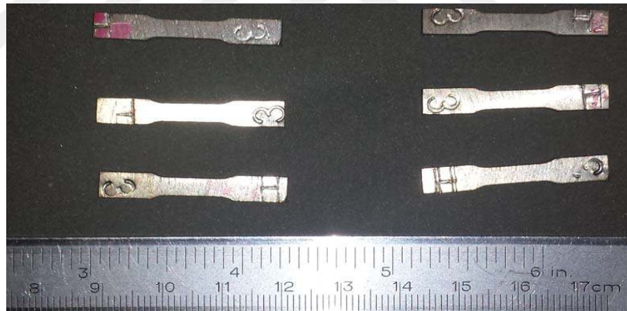
Figure E.4. Photograph illustrates the short tension specimens. Dimensions shown in Figure 3.39(b)
