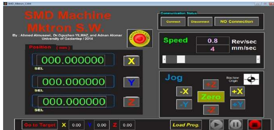
Figure 3. 34. PC-interface program (CAM) shows the amount of travel speed used (TS) = 4 mm/s.
