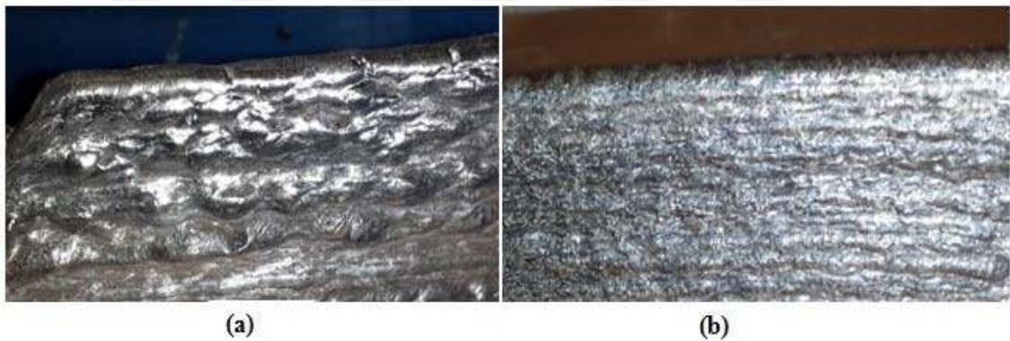
Figure 4.22. Variation in wall surface quality for (a) Experiment 9; and (b) Experiment 12.
