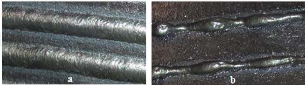
Figure 4. 15. (a) Beads of experiments 5 and 6, smooth beads ; (b) beads of experiments 19 and 20, humping beads.
