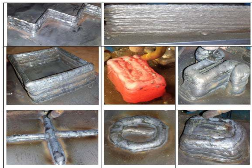
Figure 4. 2. Different solid near-net-shape deposited components using SMDM cell
