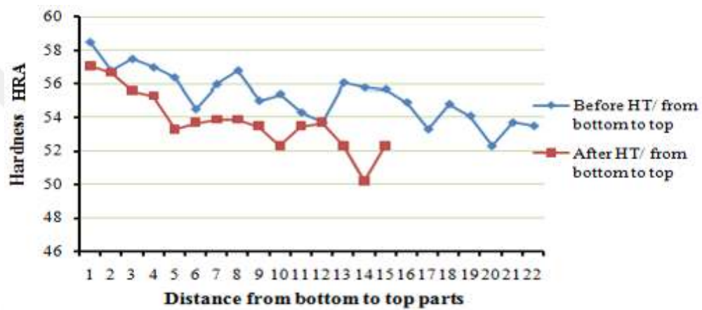
Figure 4. 89. Comparison the hardness from Bottom to the top before and after HT.
