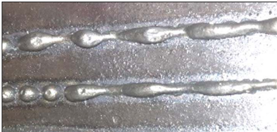
Figure 2. 19. Photograph illustrates the bead humping in TW-SMD process
