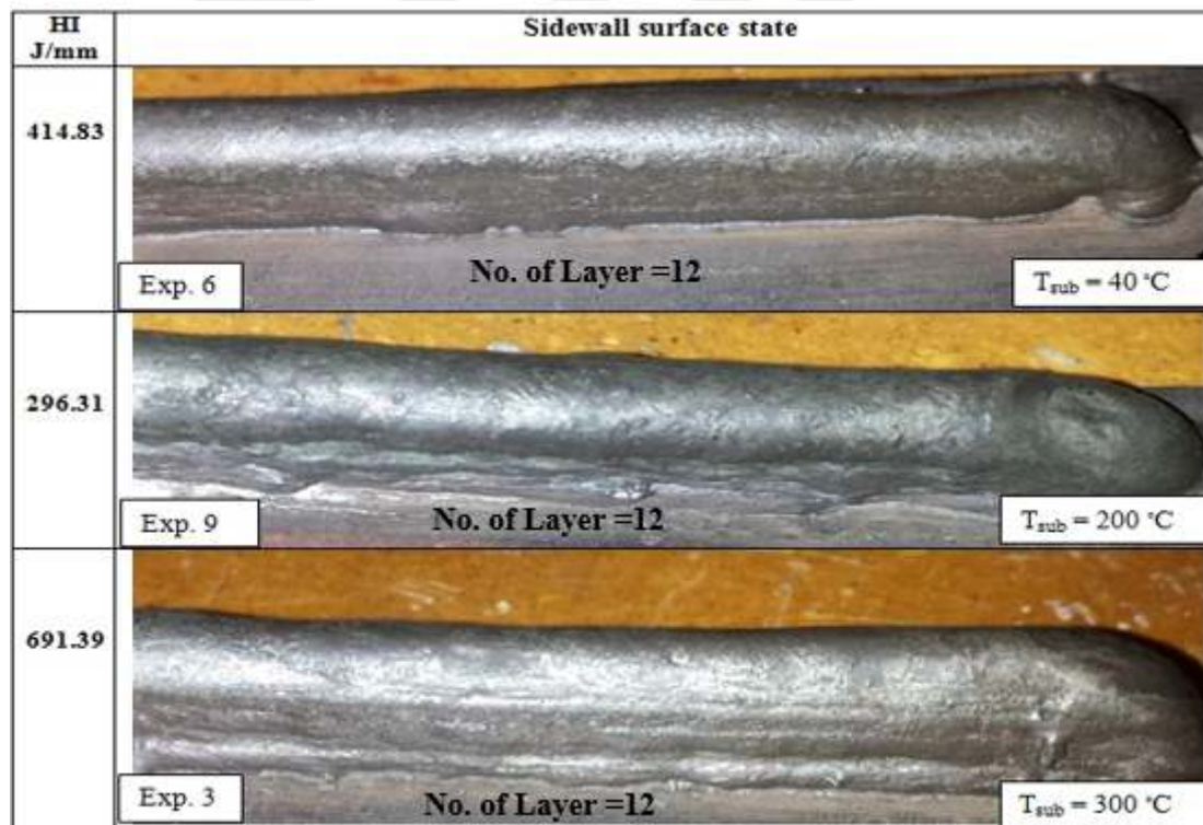
Figure 4. 31. Effects of T_{sub} and TS on the sidewall surface facet
