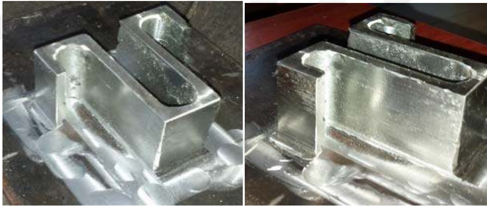
Figure 3. 37. Real deposited part after machining process
