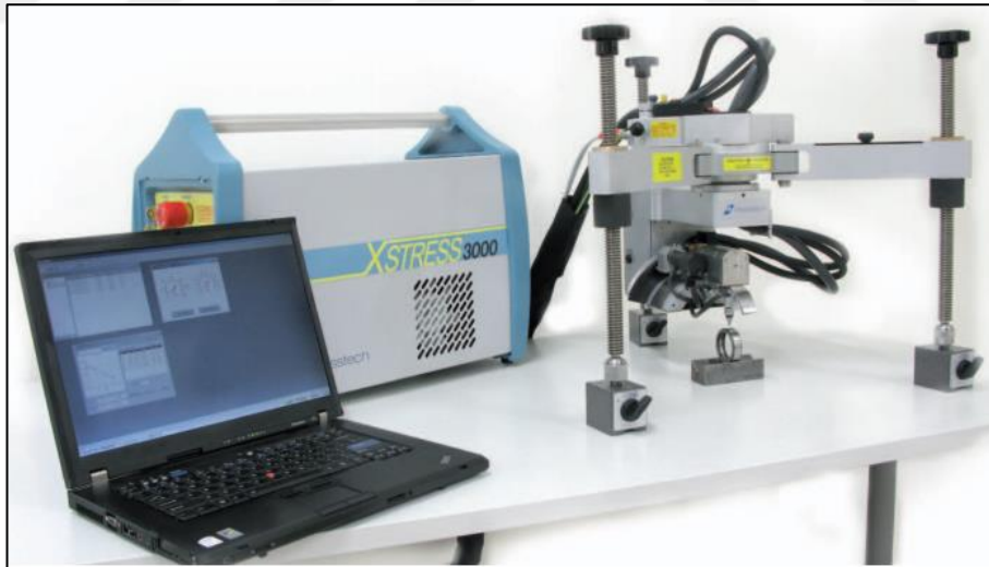
Figure 4.24 XRD residual stress measurement device [69]
