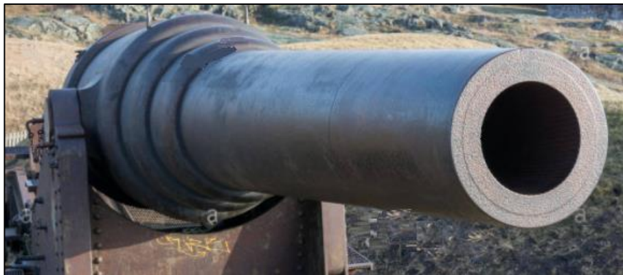
Figure 3.5 Press fitted cannon barrel [46]
