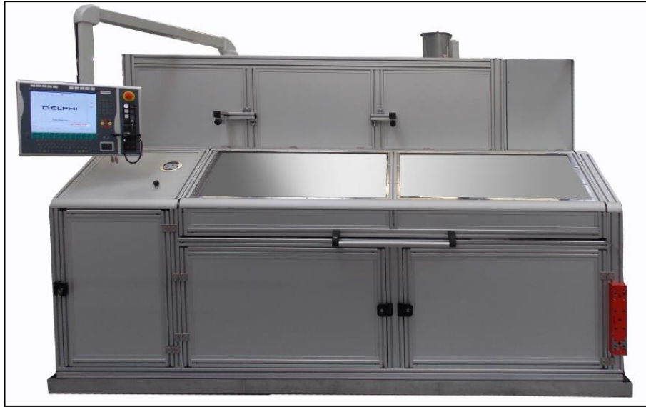
Figure 4.1 Autofrettage test unit [63]
