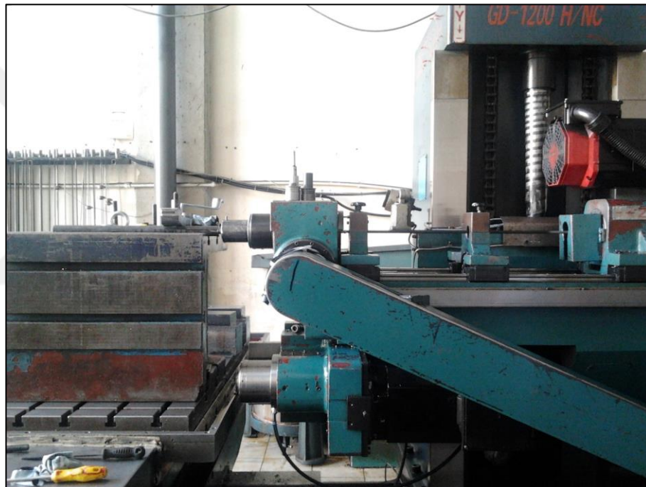
Figure 4.7 Gun drilling process [64]
