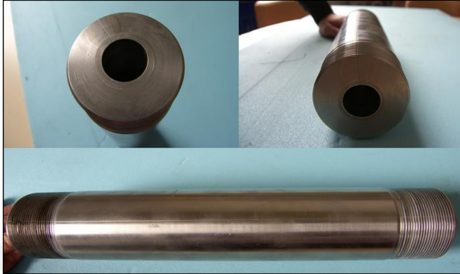
Figure 3.4 Failure on a high pressure cylinder of an intensifier pump [45]
