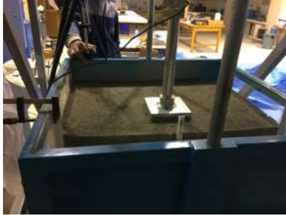
Figure 4.14. Placing the foundation
