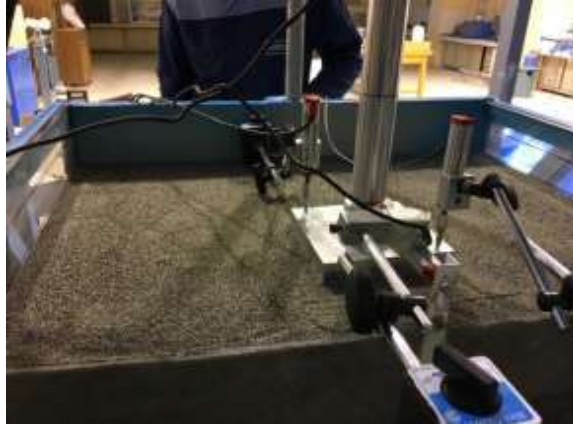
Figure 4.17. Setting the lvdt
