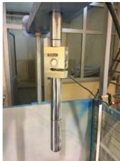
Figure 4.4. Hydraulic load system and load cell
