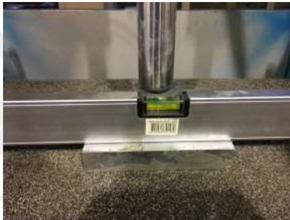
Figure 4.15. Foundation leveling control -1
